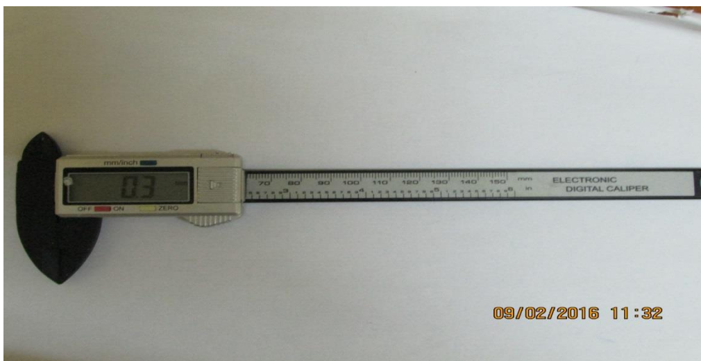
Figure 2: Digital Vernier Caliper: Instrument that was used to measure external diameter of the PcoA
