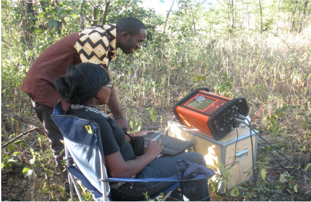
Figure 19: WalkTEM equipment being used during TDEM soundings in the Machile River Basin, South-Western Zambia
