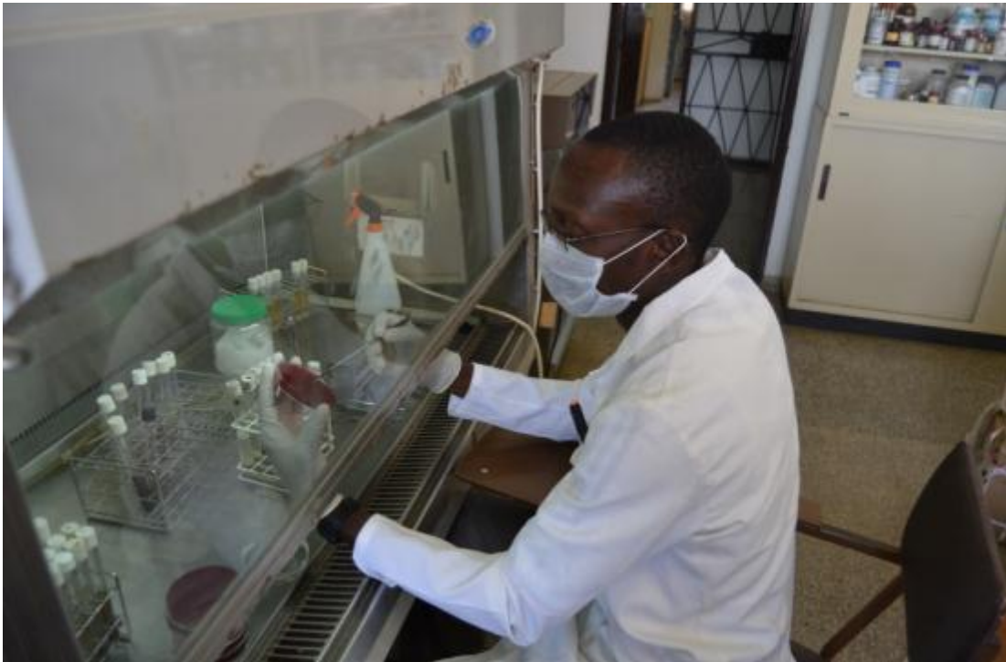
Figure 3.4: Activated samples being inoculated under the biosafety cabinet.
