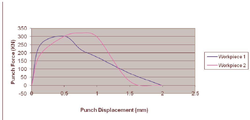
Figure 4.15: Comparison of Blanking Forces
