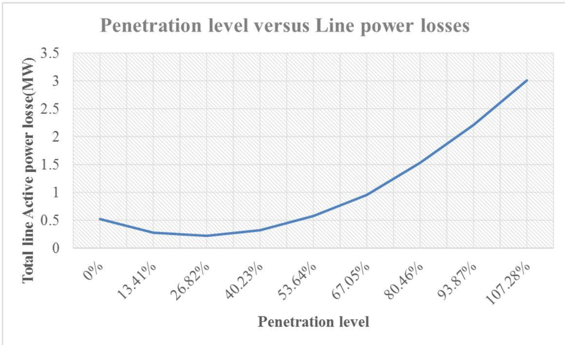
**Figure 23:** Penetration level versus Power losses at Makeni substation
