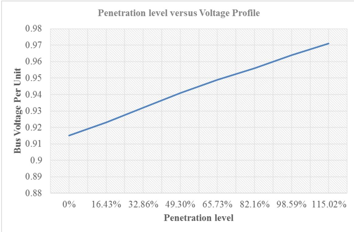
**Figure 51:** Penetration level versus Voltage profile at Chawama substation
