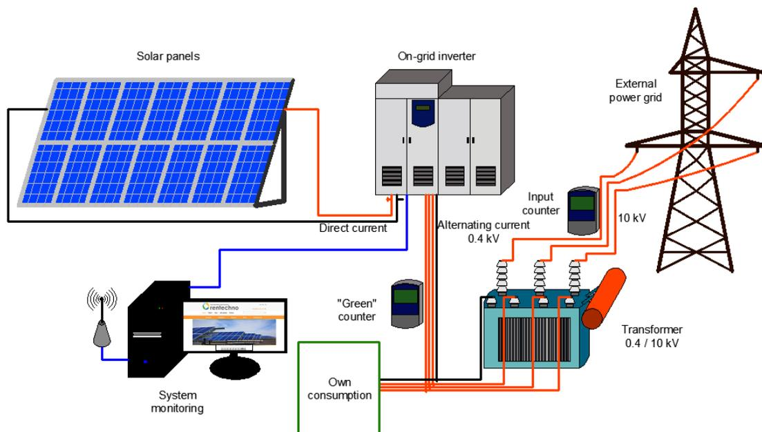
**Figure 7:** Typical grid connected centralized PV (Rentechno Group, 2009)
