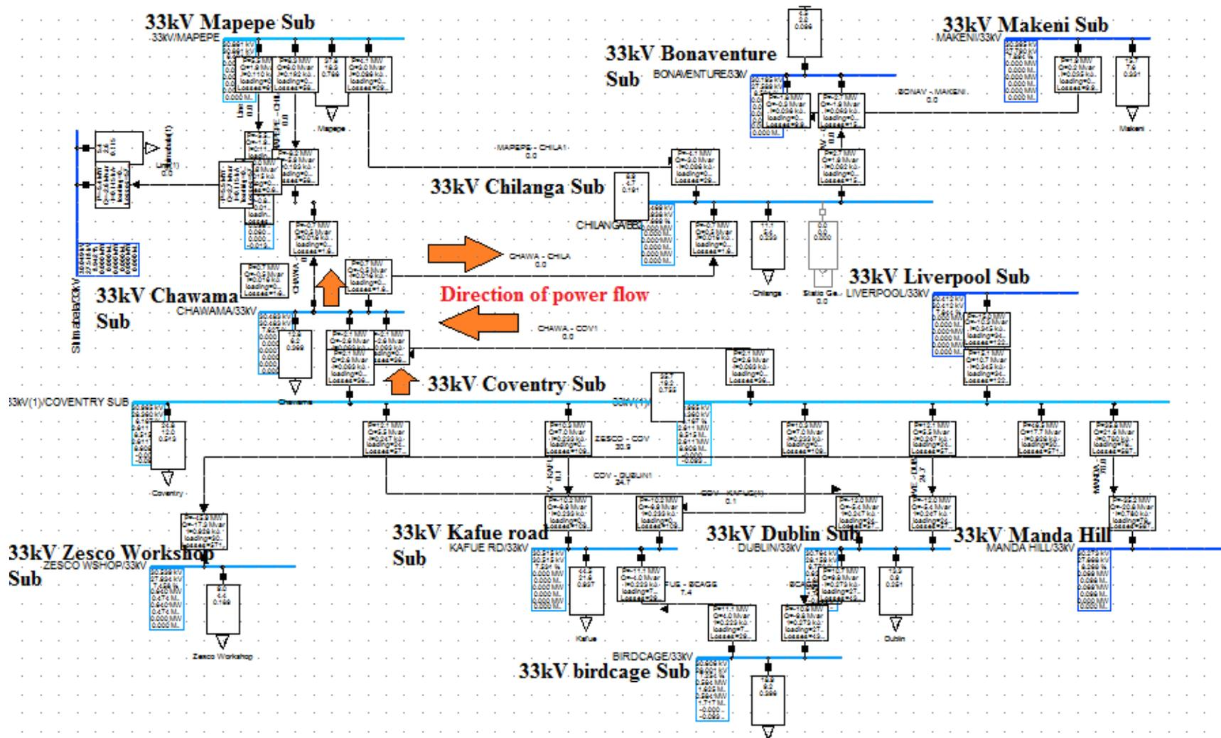
Figure 53: Intial Power flow direction change after a 16.43% (10MW) solar PV plant connection at Chawama substation
