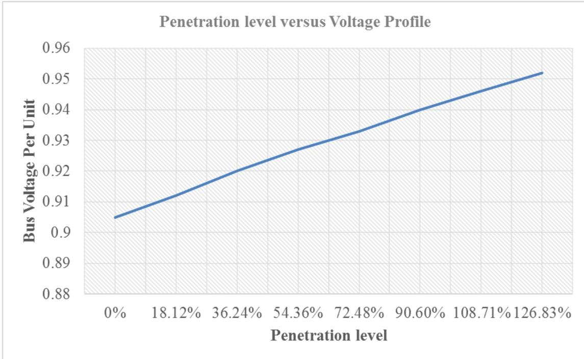
**Figure 33:** Penetration level versus Voltage profile impact at Avondale substation
