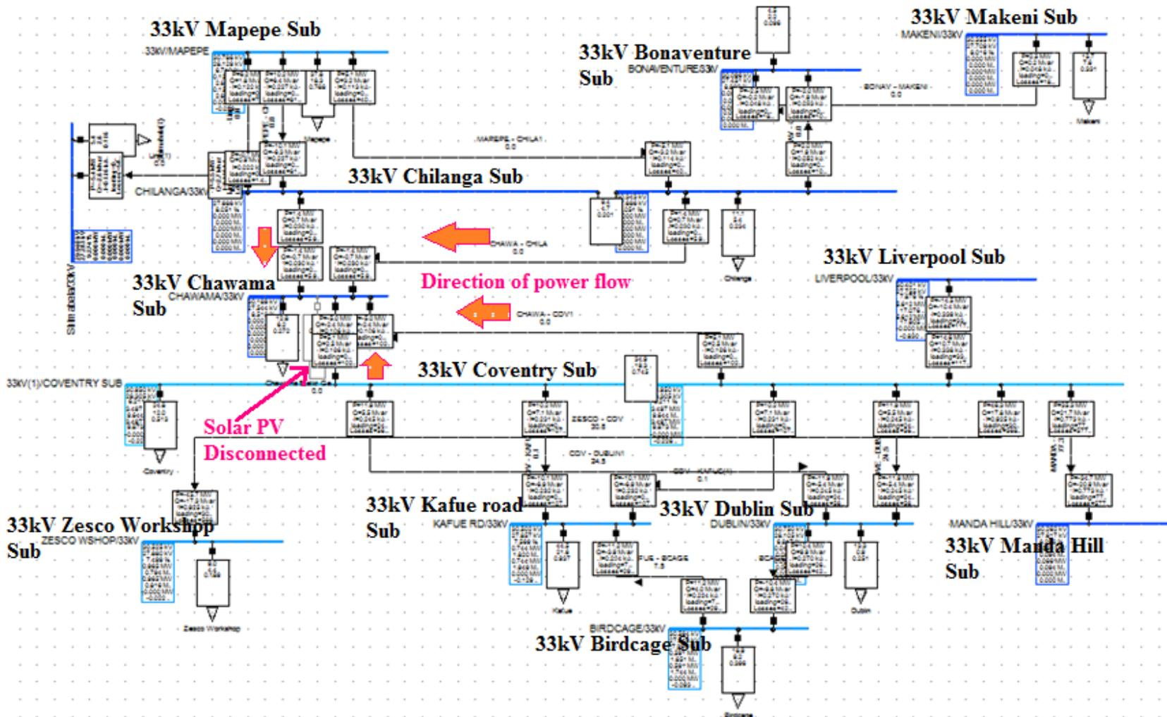
Figure 52: Power flow direction before solar PV plant connection at Chawama substation
