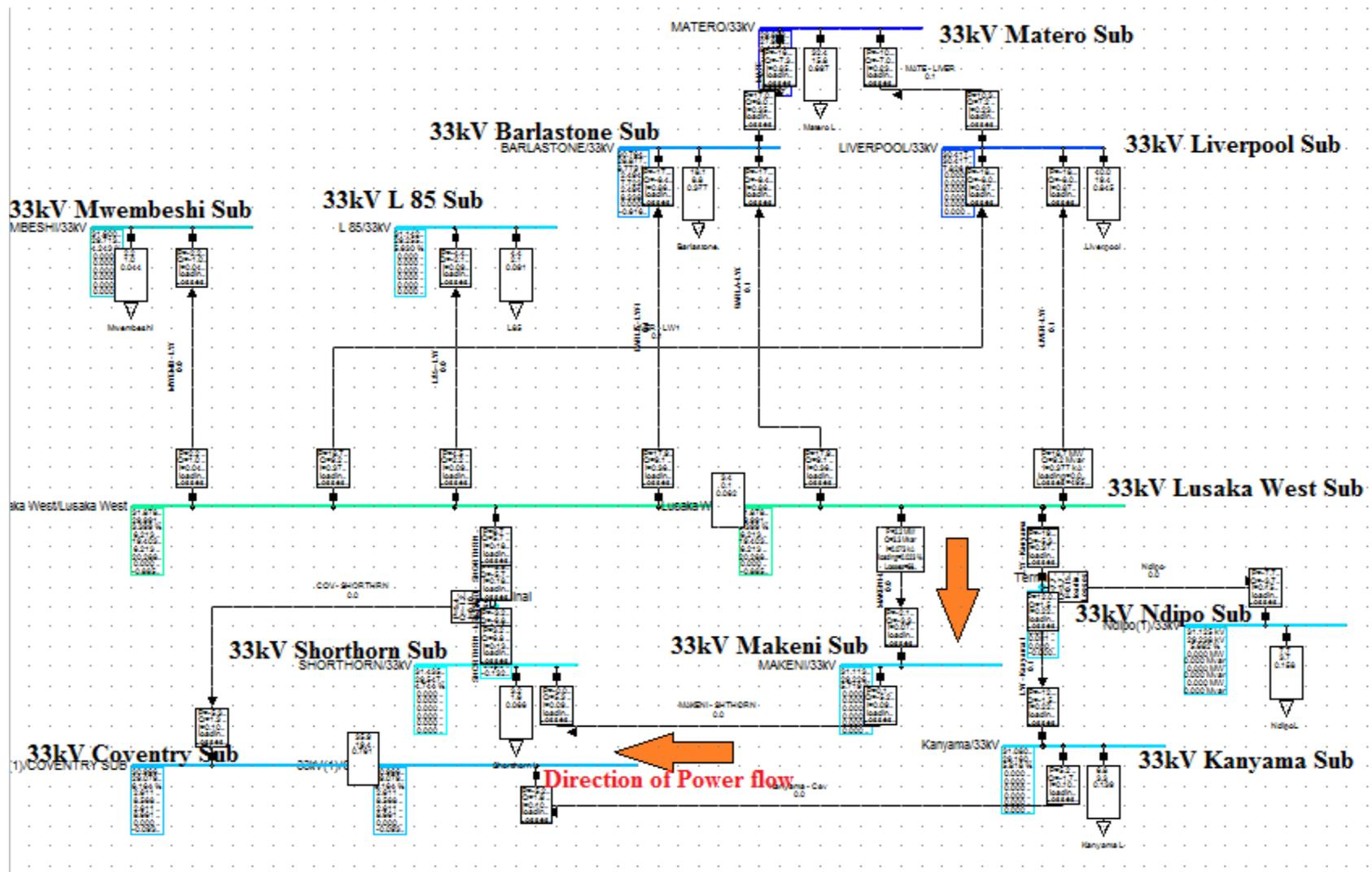
**Figure 26** Initial Power flow direction change after a 26.82% (20MW) solar PV plant connection at Makeni substation
