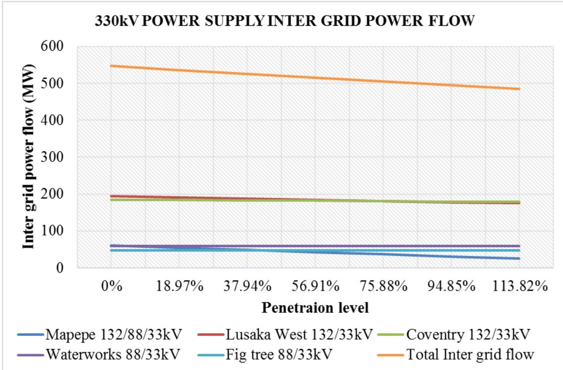
**Figure 65:** 330kV supply inter grid power flow impact due to integration a Chilanga substation
