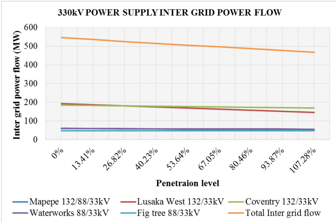
**Figure 29:** 330kV supply inter grid power flow impact due to integration at Makeni substation
