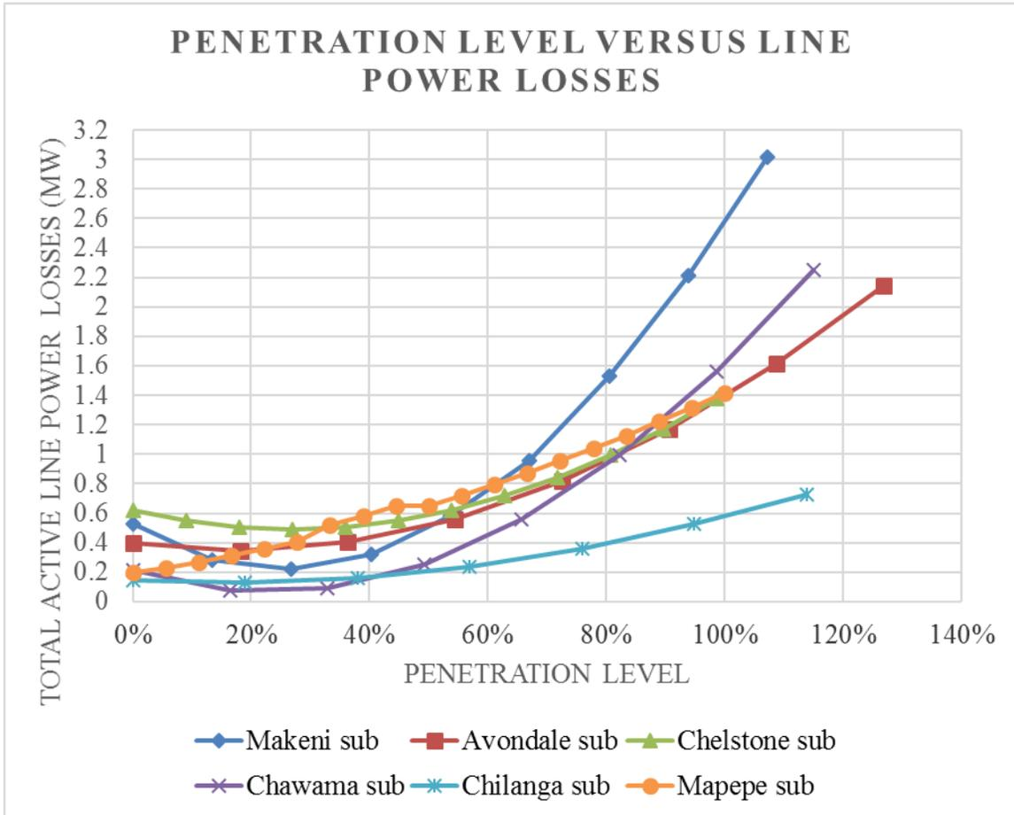
**Figure 76:** Penetration level versus line power losses analysis for the six substations
