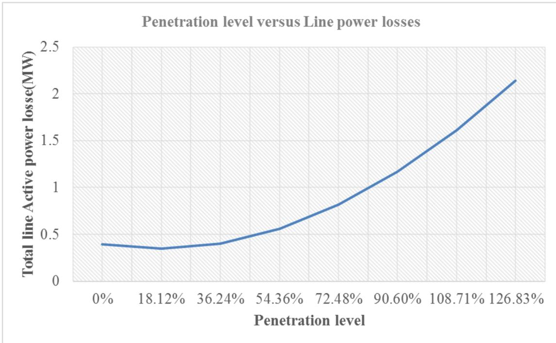
**Figure 32:** Penetration level versus Power losses impact at Avondale substation
