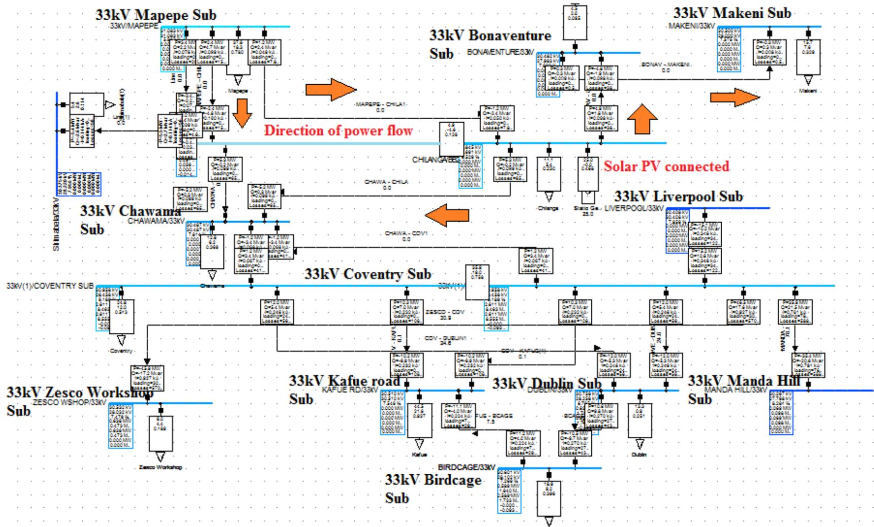
Figure 62: Initial Power flow change direction after a 47.335% (25MW) solar PV plant connection at Chilanga substation
