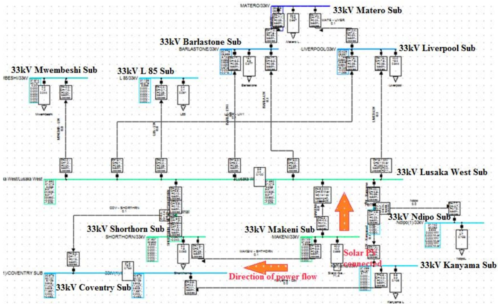
**Figure 27:** Overall Power flow direction change after a 67.05% (50MW) solar PV plant connection at Makeni substation
