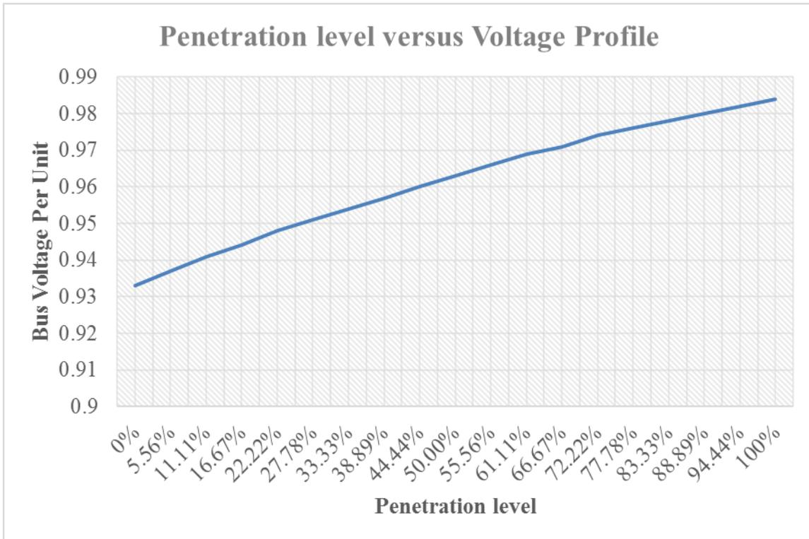
**Figure 69:** Penetration level versus Voltage profile at Mapepe substation
