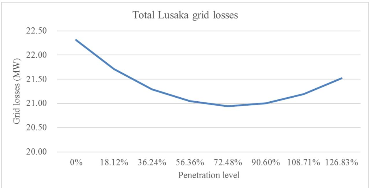
**Figure 40:** Total Lusaka network grid losses impact due to integration at Avondale substation
