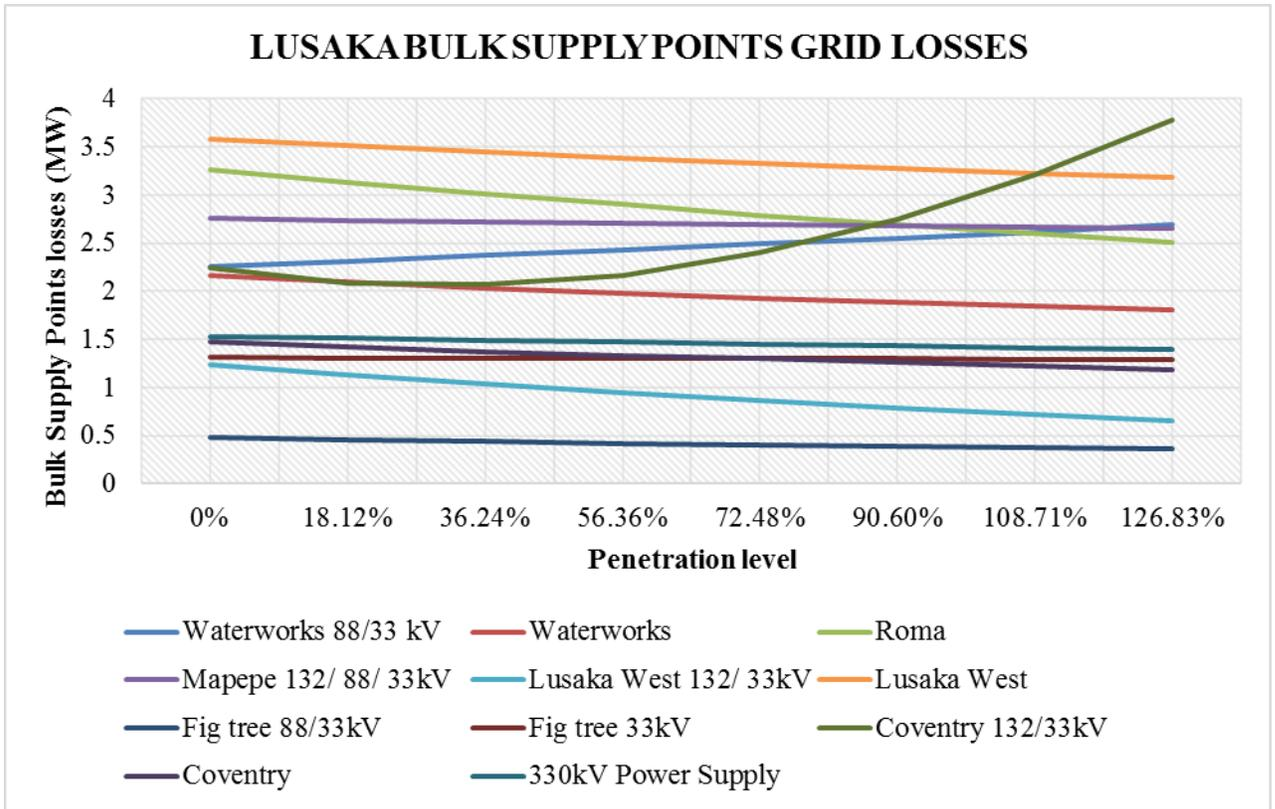
**Figure 39:** Lusaka bulk supply points grid losses impact due to integration at Avondale substation
