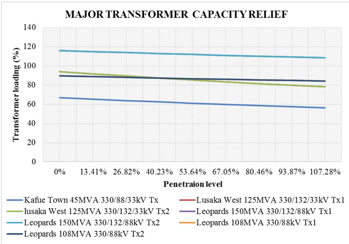
**Figure 28:** Major transformer capacity relief due integration at Makeni substation
