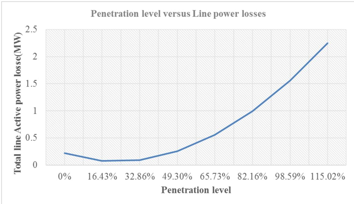
**Figure 50:** Penetration level versus Power losses at Chawama substation
