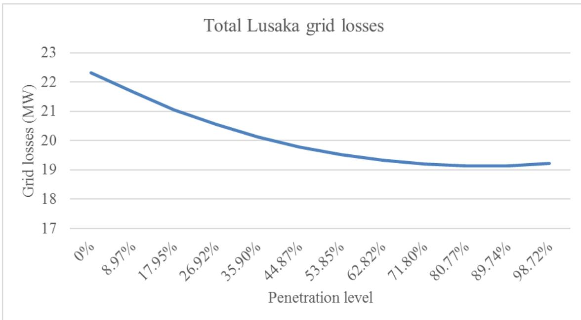
**Figure 49:** Lusaka network grid losses impact due to integration at Chelstone substation
