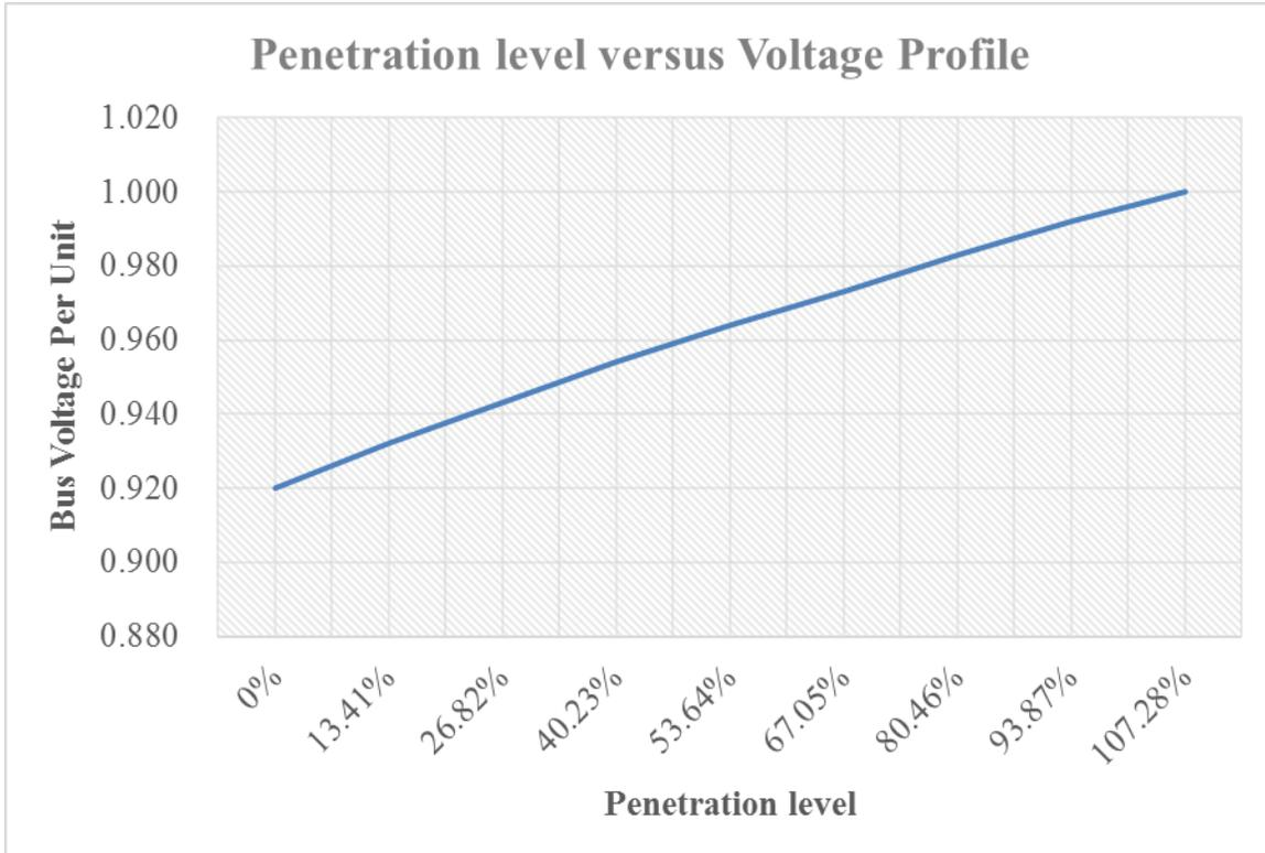
**Figure 24:** Penetration level versus Voltage profile at Makeni substation
