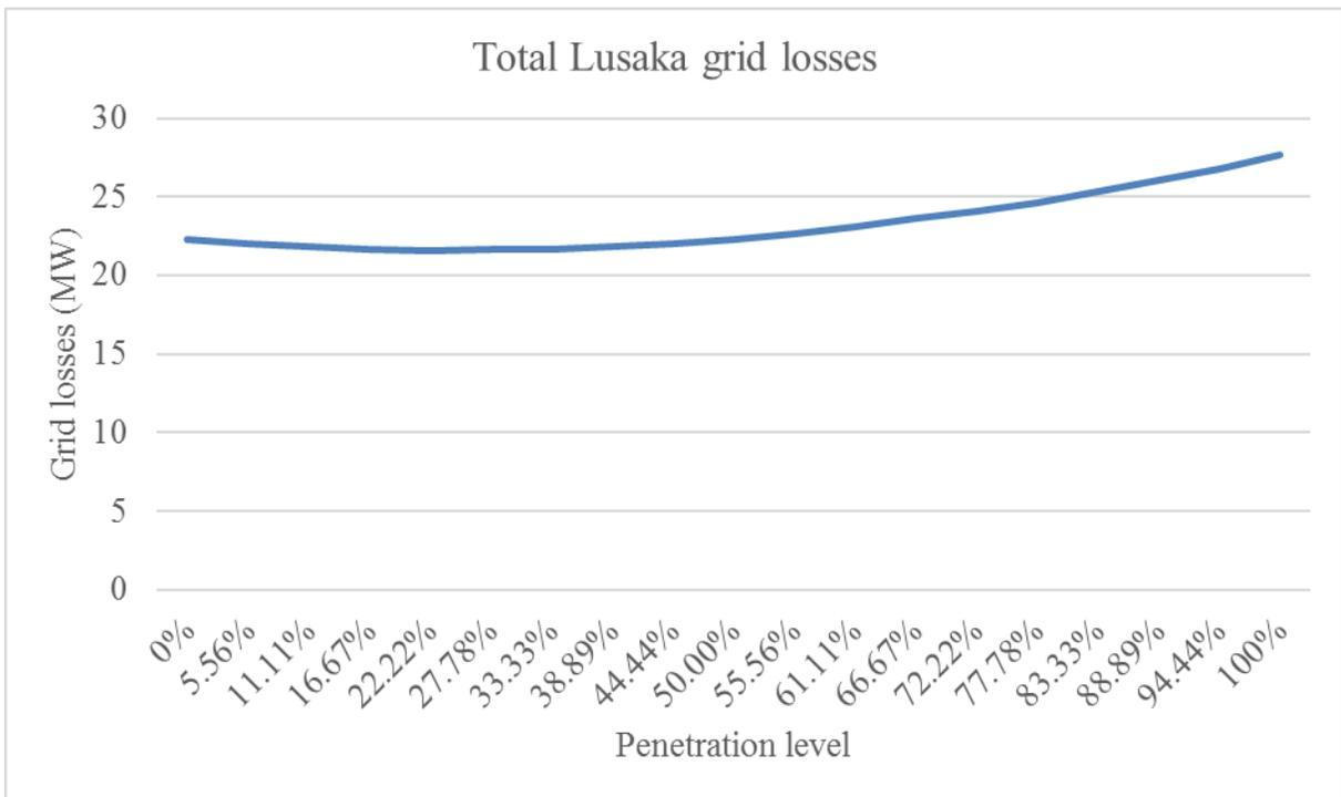
**Figure 75:** Lusaka network grid losses impact due to integration at Mapepe substation
