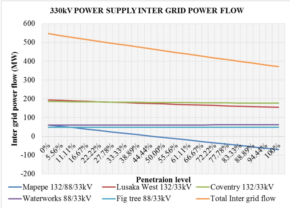
**Figure 73:** 330kV supply inter grid power flow impact due to integration at Mapepe substation
