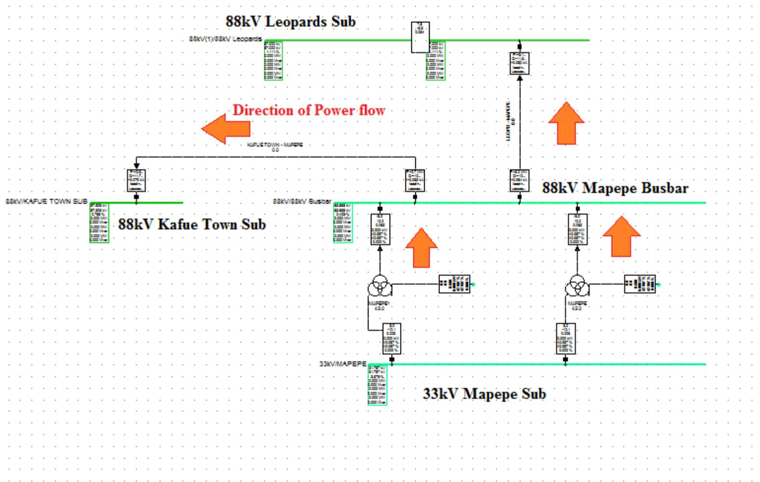
**Figure 71:** Initial and overall Power flow direction change after a 50.00% (90MW) solar PV plant connection at Mapepe substation
