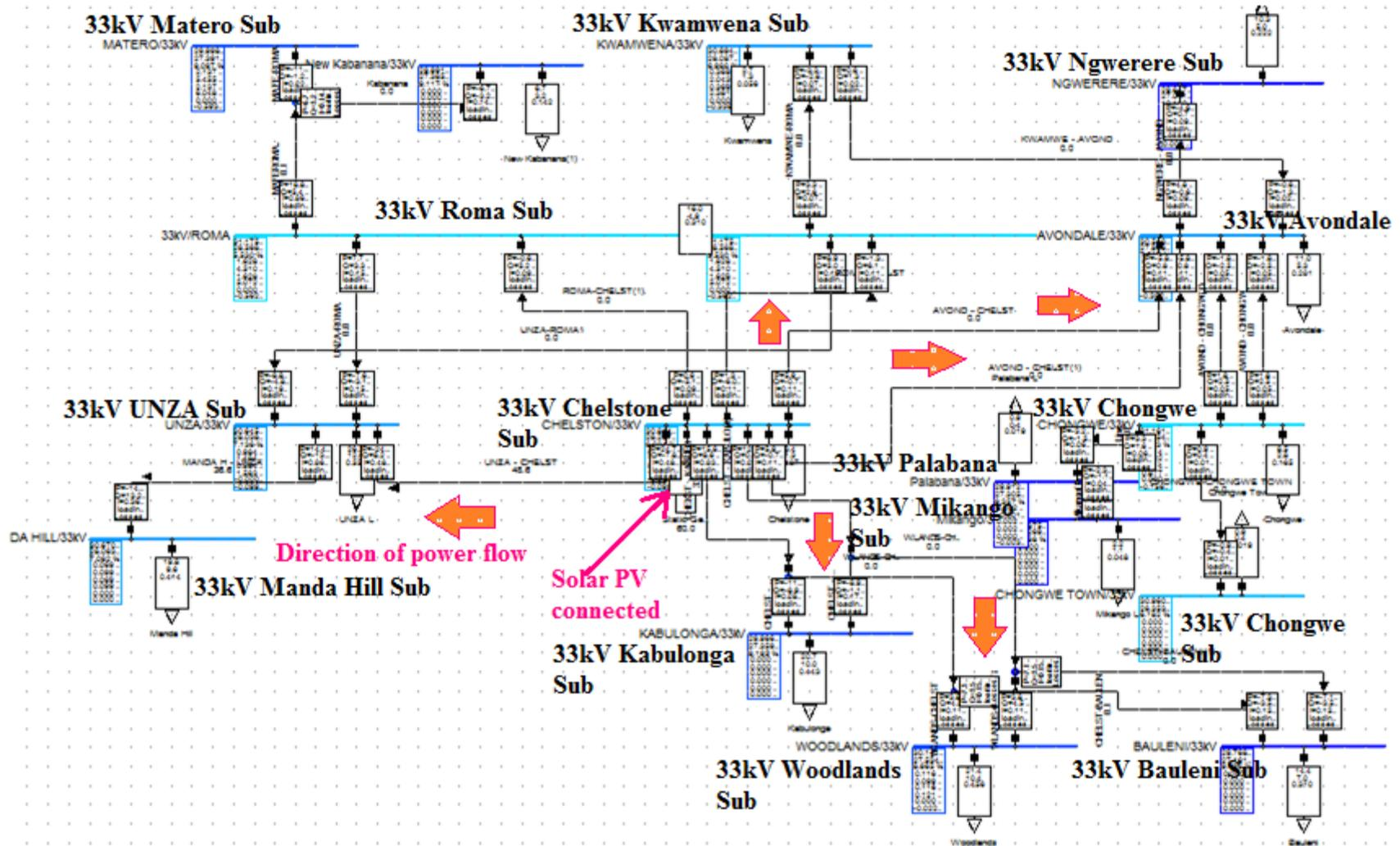
**Figure 45:** Overall Power flow direction change after a 80.77% (90MW) solar PV plant connection at Chelstone substation
