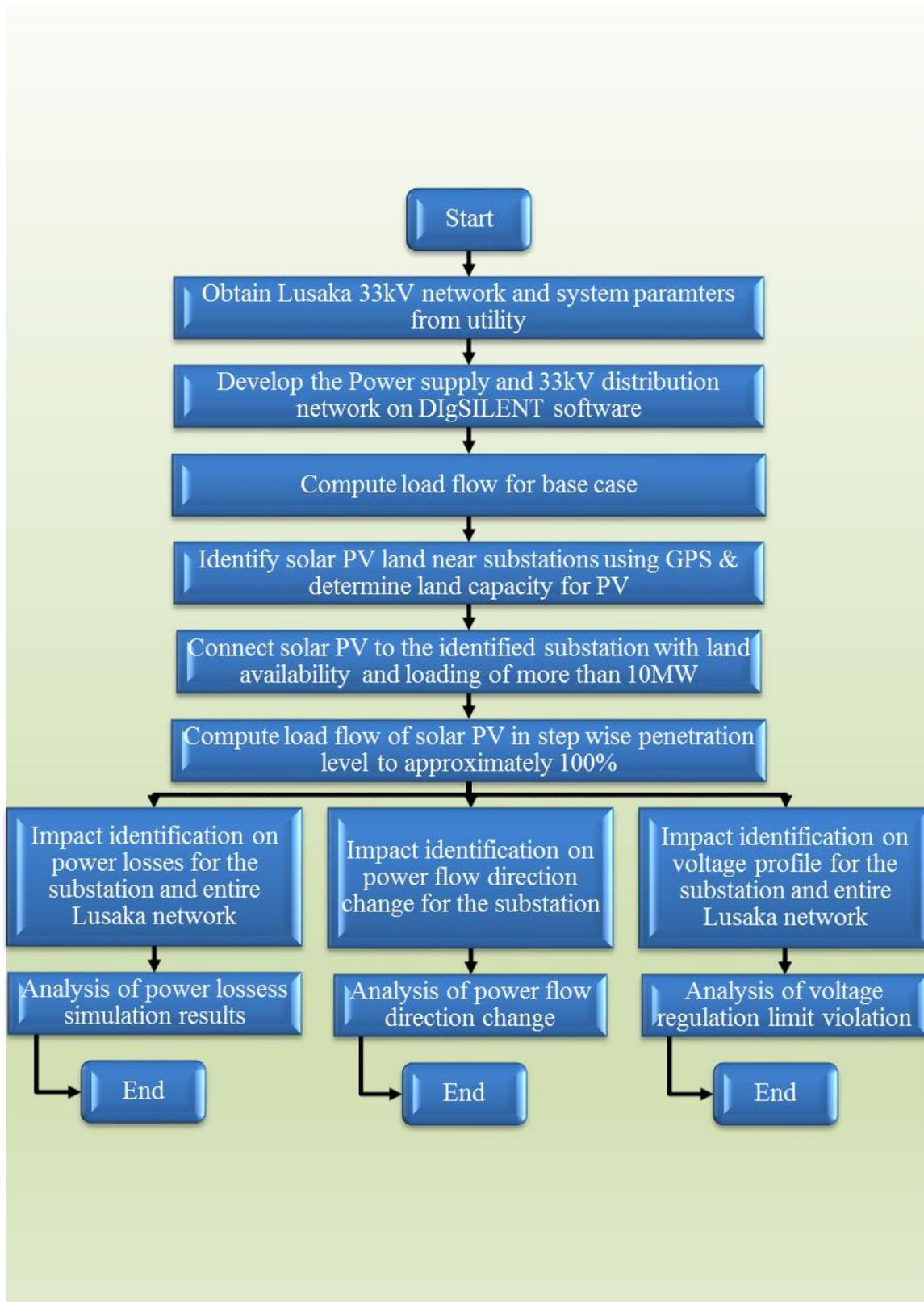
**Figure 8:** System methodology flow chart
