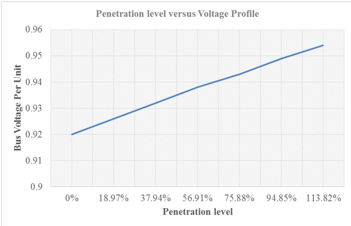
**Figure 60:** Penetration level versus Voltage profile at Chilanga substation
