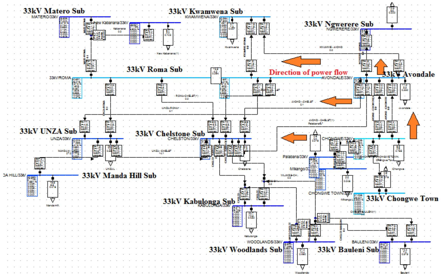
**Figure 35:** Initial Power flow direction change after a 54.36% (30MW) solar PV plant connection at Avondale substation
