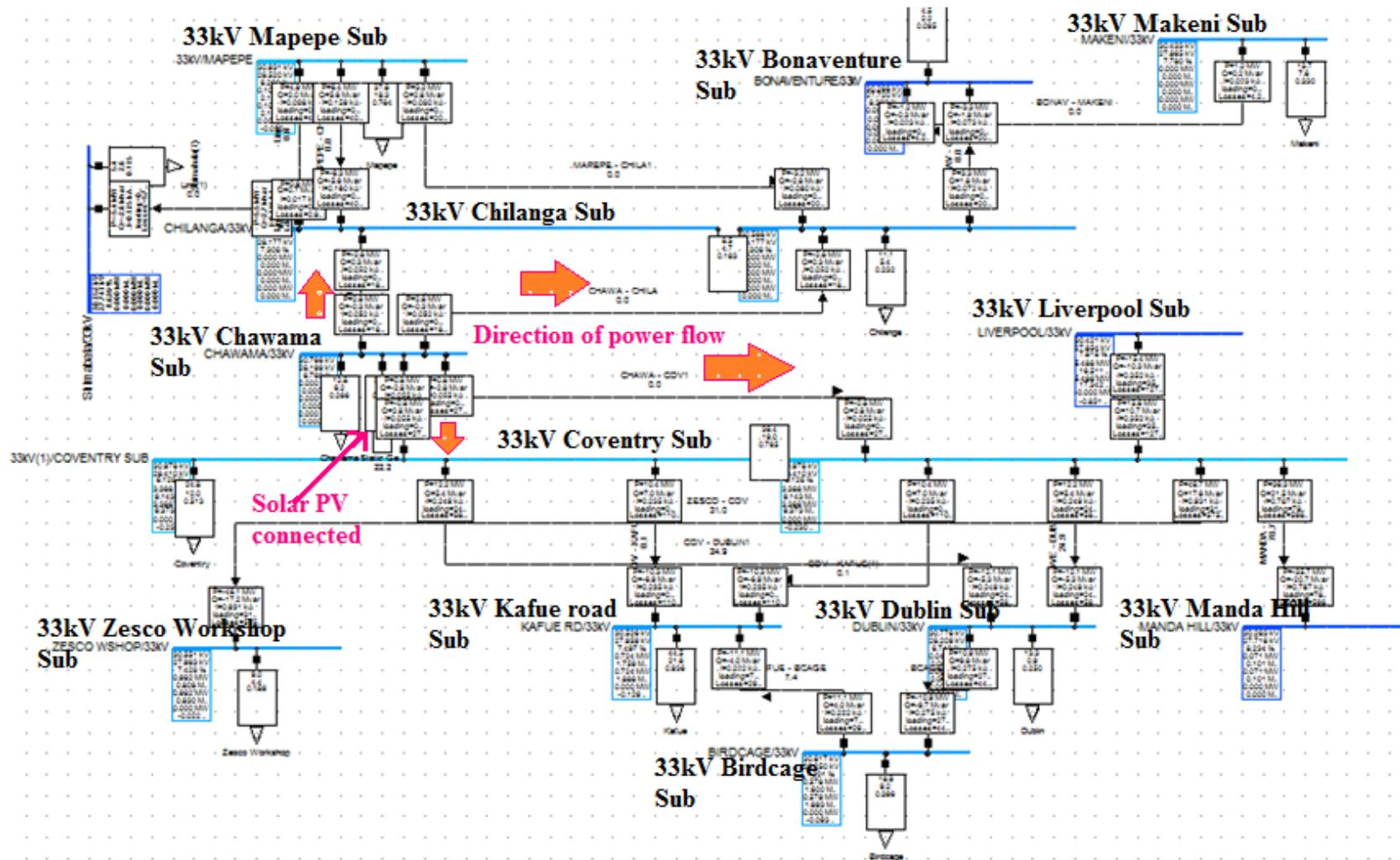
**Figure 54:** Overall Power flow direction change after a 32.86% (20MW) solar PV plant connection at Chawama substation
