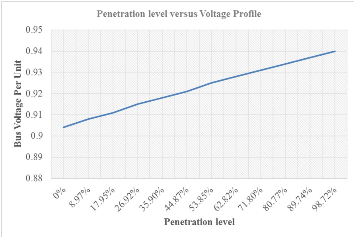
**Figure 42:** Penetration level versus Voltage profile at Chelstone substation
