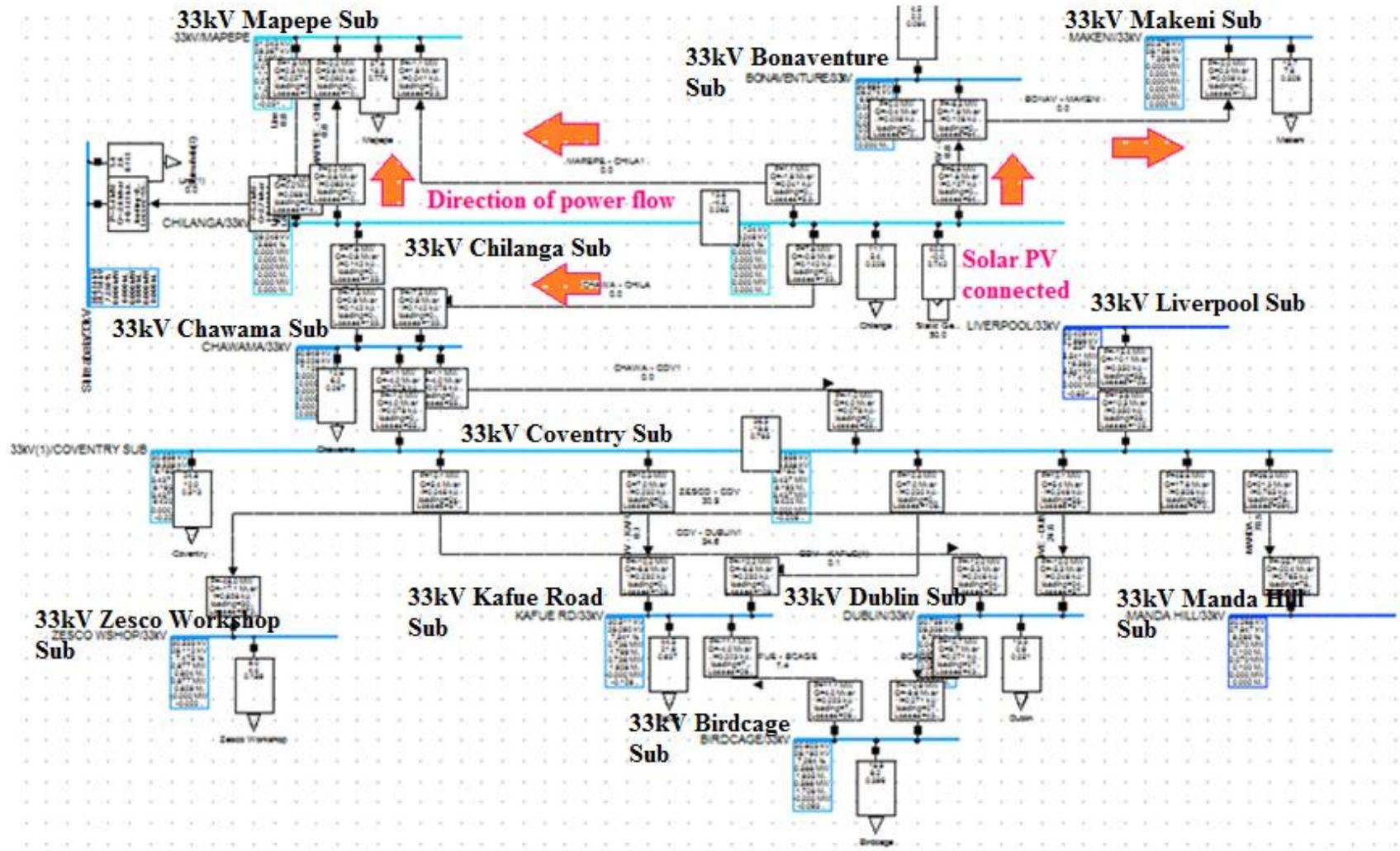
**Figure 63:** Overall Power flow change direction after a 75.88% (40MW) solar PV plant connection at Chilanga substation
