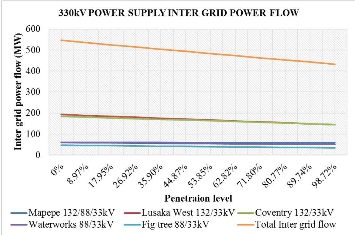
**Figure 47:** 330kV supply inter grid power flow impact due to integration at Chelstone substation
