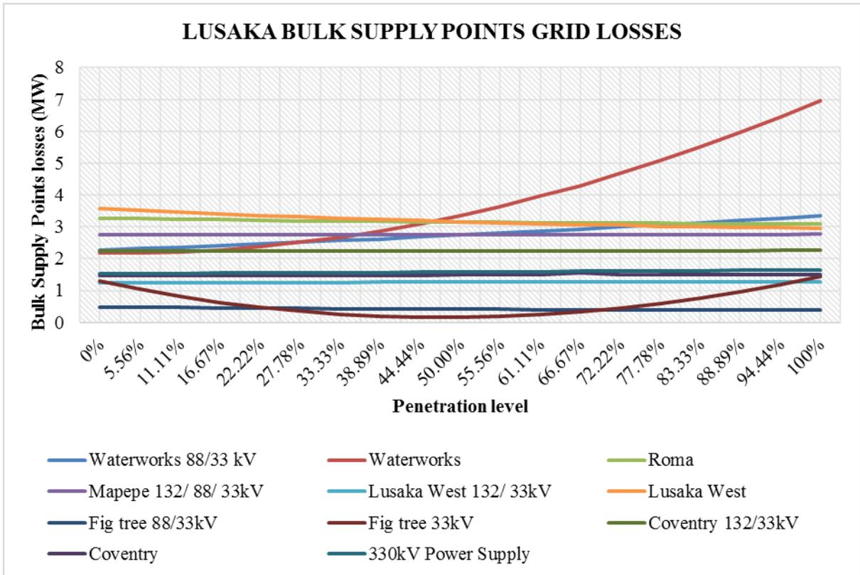
**Figure 74:** Lusaka bulk supply points grid losses impact due to integration at Mapepe substation
