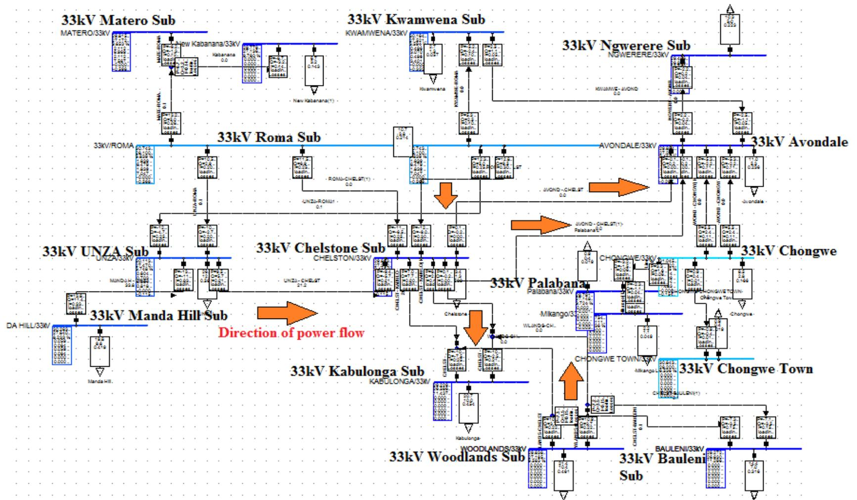
**Figure 44:** Initial Power flow direction change after a 4.485% (5MW) solar PV plant connection at Chelstone substation
