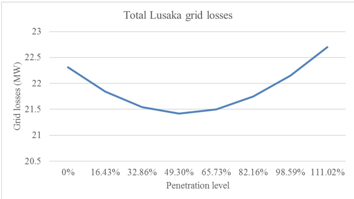
**Figure 58:** Lusaka network grid losses impact due to integration at Chawama substation
