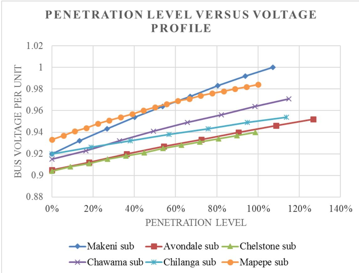
**Figure 77:** Penetration level versus voltage profile analysis for the six substations
