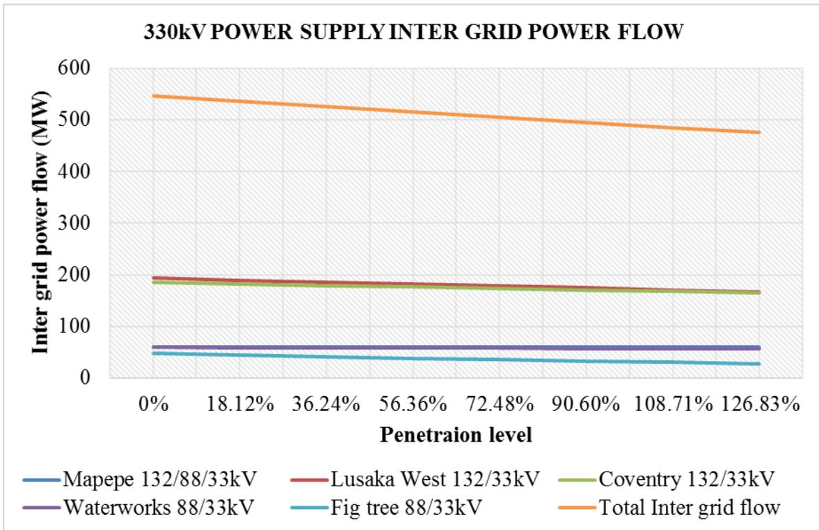
**Figure 38:** 330kV supply inter grid power flow impact due to integration at Avondale substation
