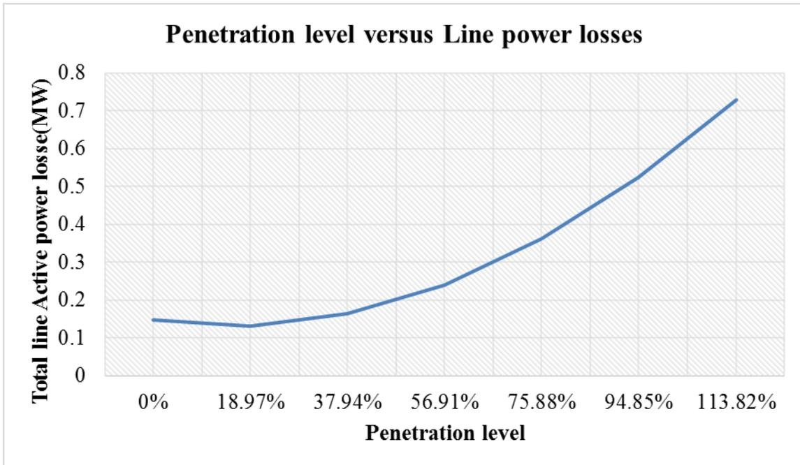
**Figure 59:** Penetration level versus Power losses at Chilanga substation
