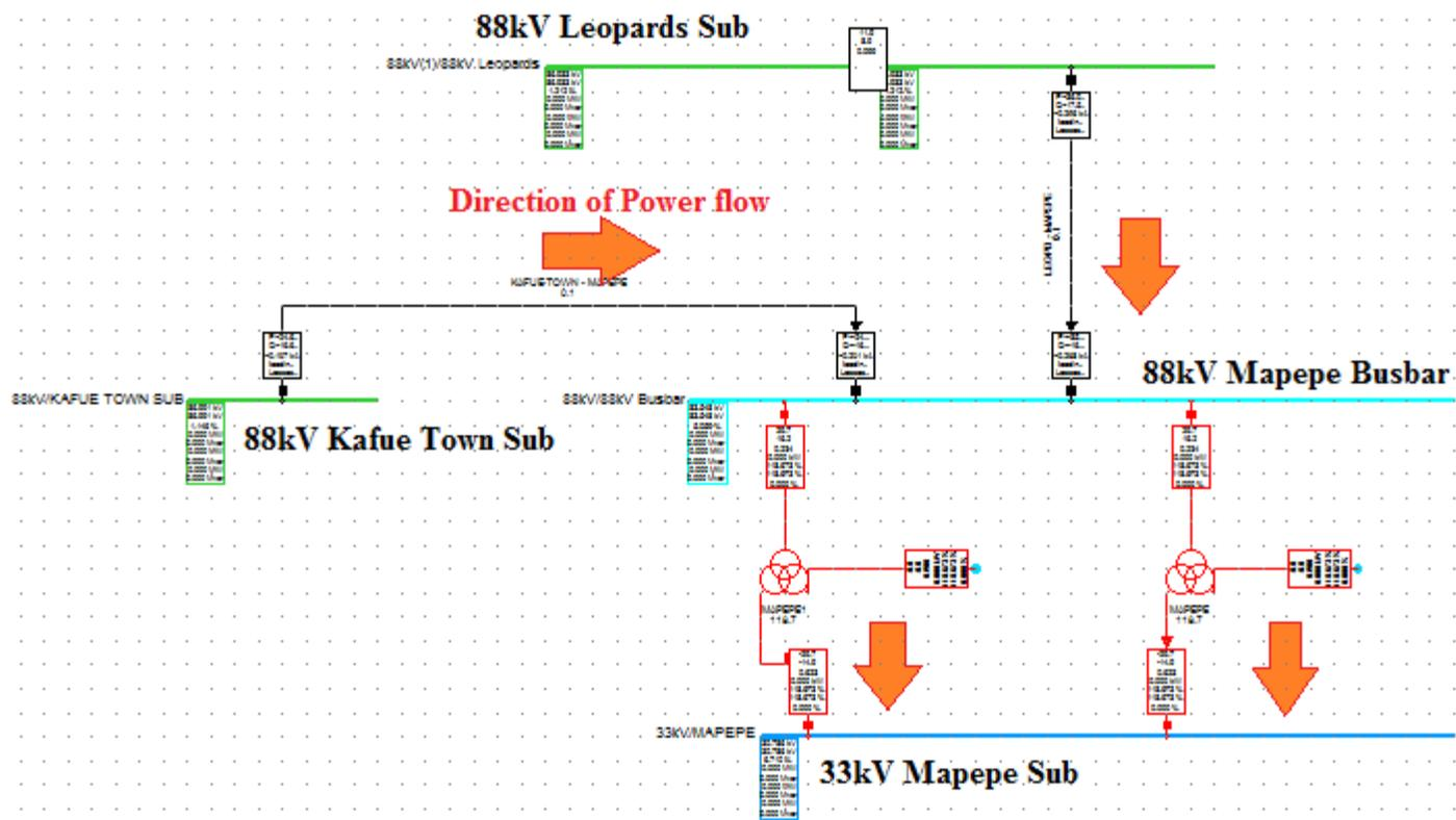
**Figure 70:** Power flow direction before solar PV plant connection at Mapepe substation
