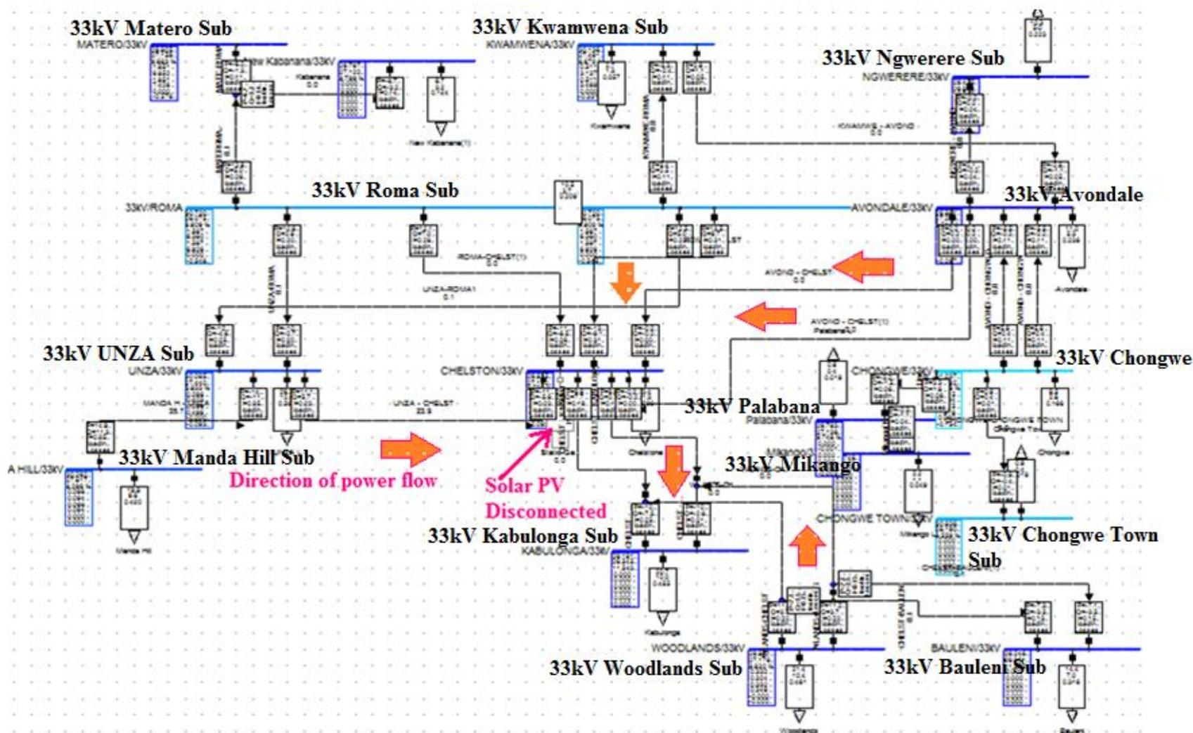
Figure 43: Power flow direction before solar PV plant connection at Chelstone substation
