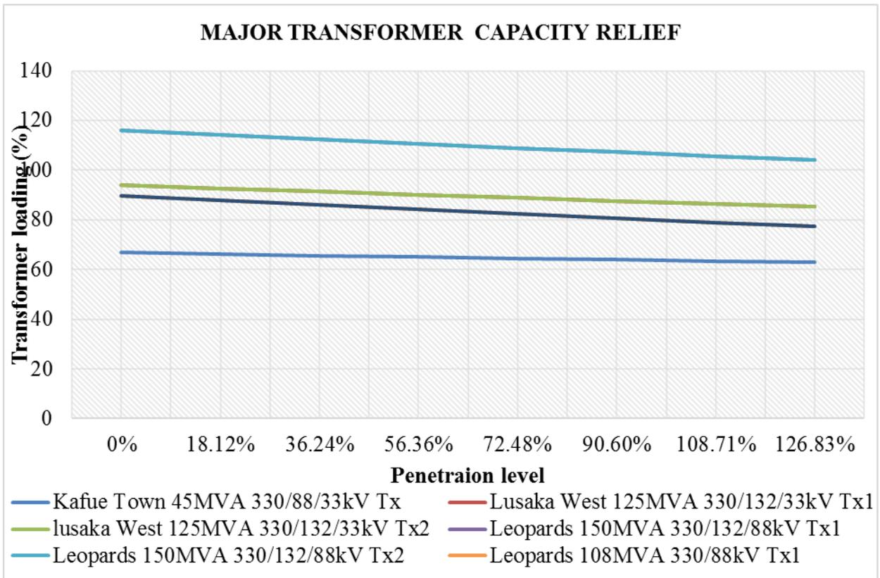
**Figure 37:** Major transformer capacity relief impact due to integration at Avondale substation
