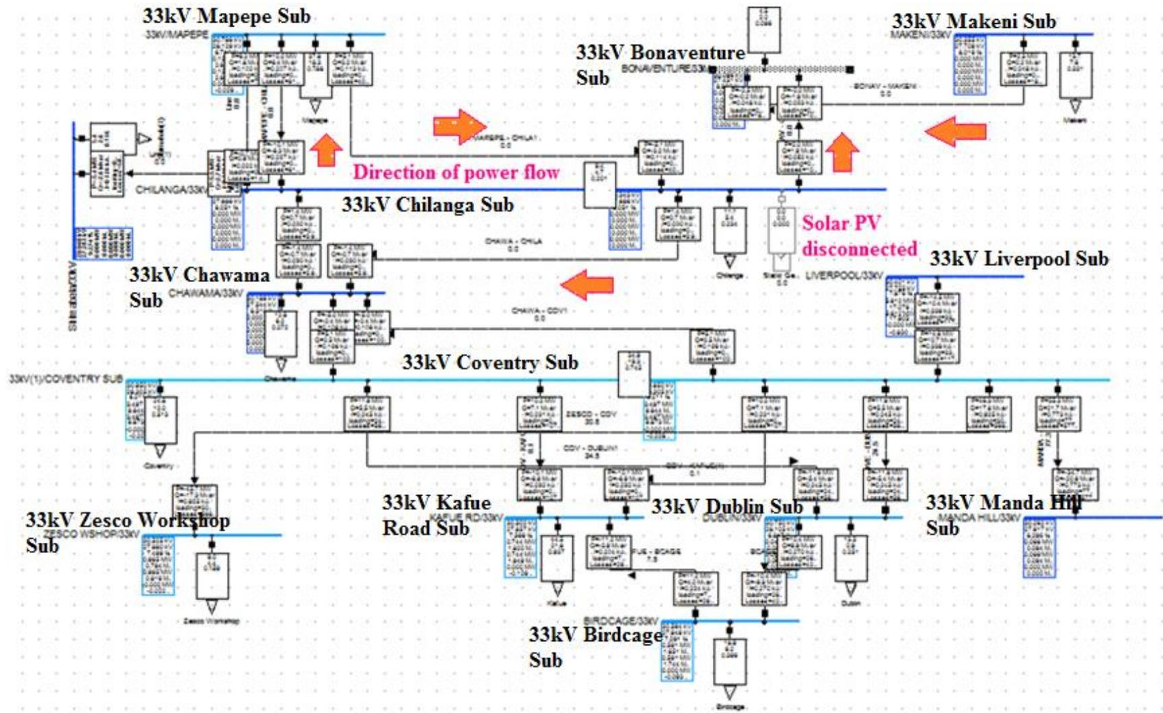
Figure 61: Power flow direction before solar PV plant connection at Chilanga substation
