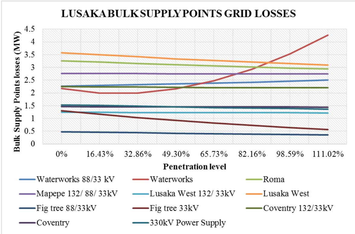
**Figure 57:** Lusaka bulk supply points grid losses impact due to integration at Chawama substation
