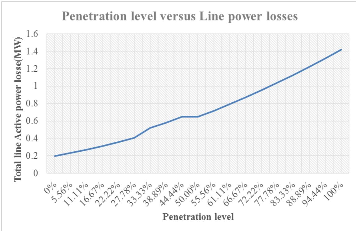
**Figure 68:** Penetration level versus Power losses at Mapepe substation
