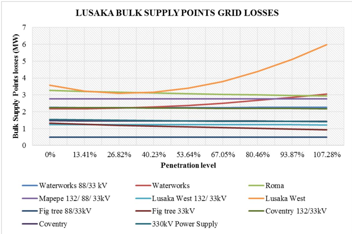
**Figure 30:** Lusaka bulk supply points grid losses impact due to integration at Makeni substation
