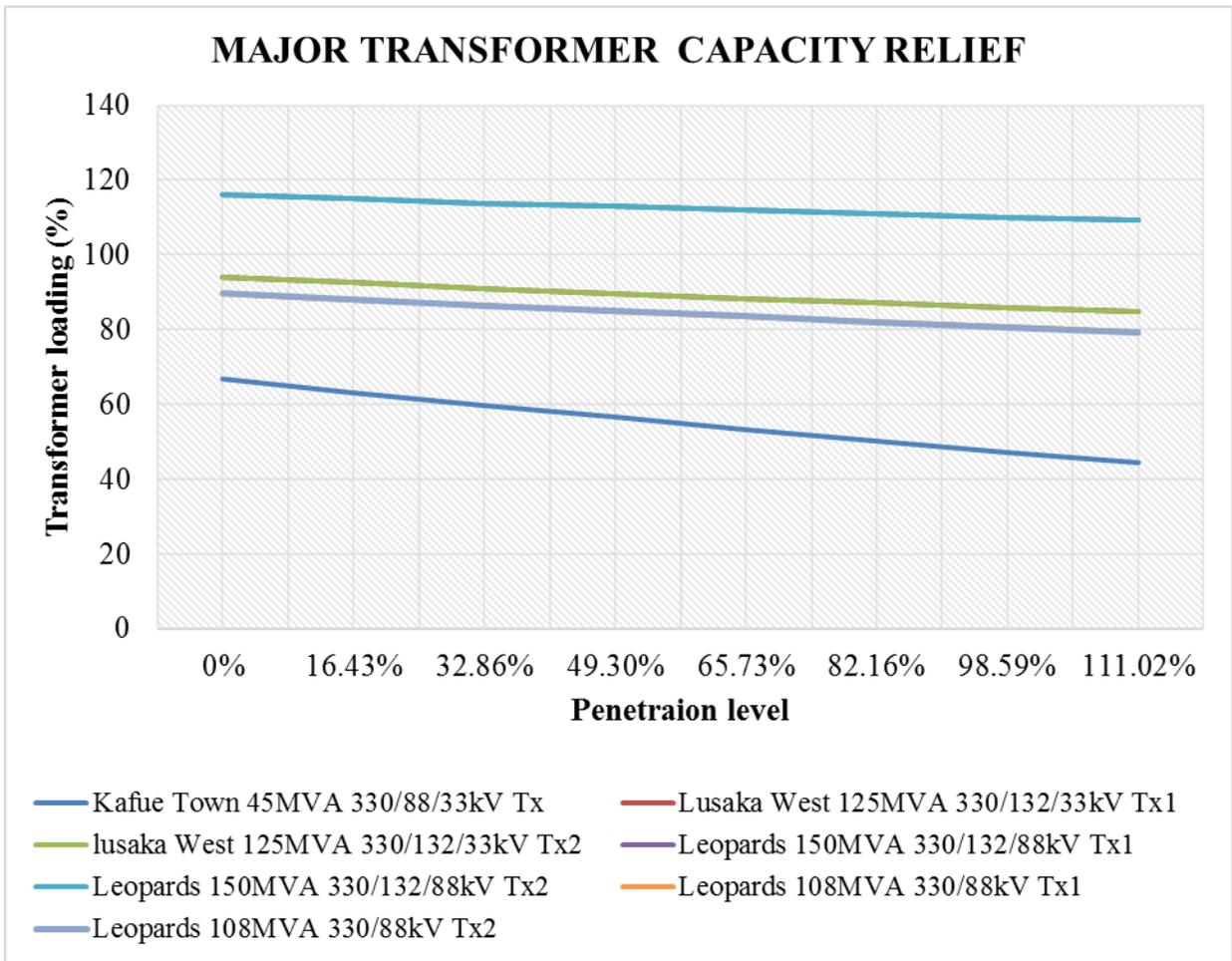
**Figure 55:** Major transformer capacity relief impact due to integration at Chawama substation
