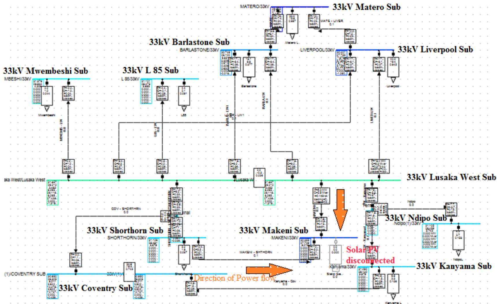
Figure 25: Power flow direction before solar PV plant connection at Makeni substation
