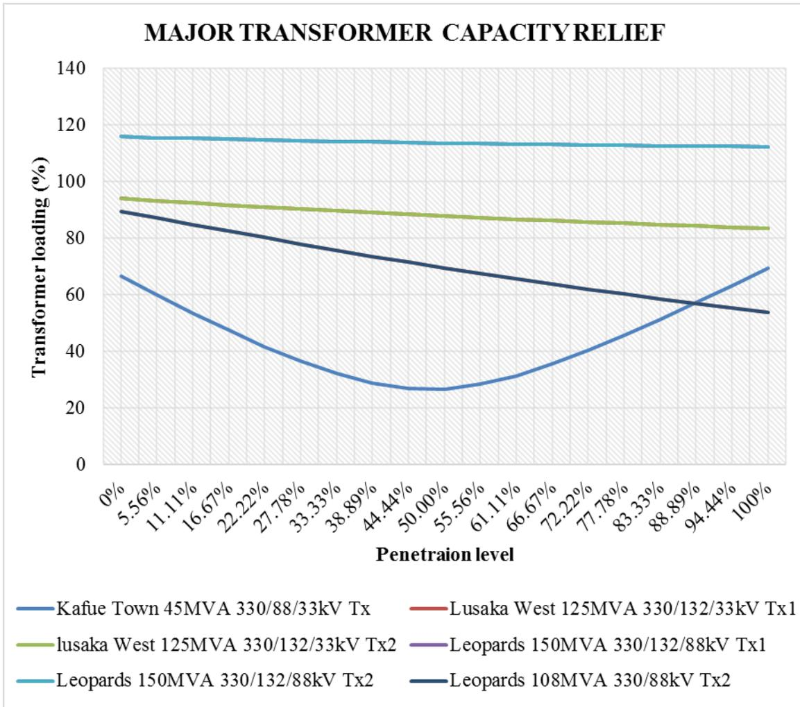
**Figure 72:** Major transformer capacity relief impact due to integration at Mapepe substation
