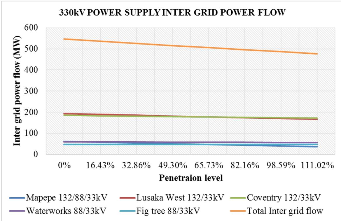
**Figure 56:** 330kV supply inter grid power flow impact due to integration at Chawama substation
