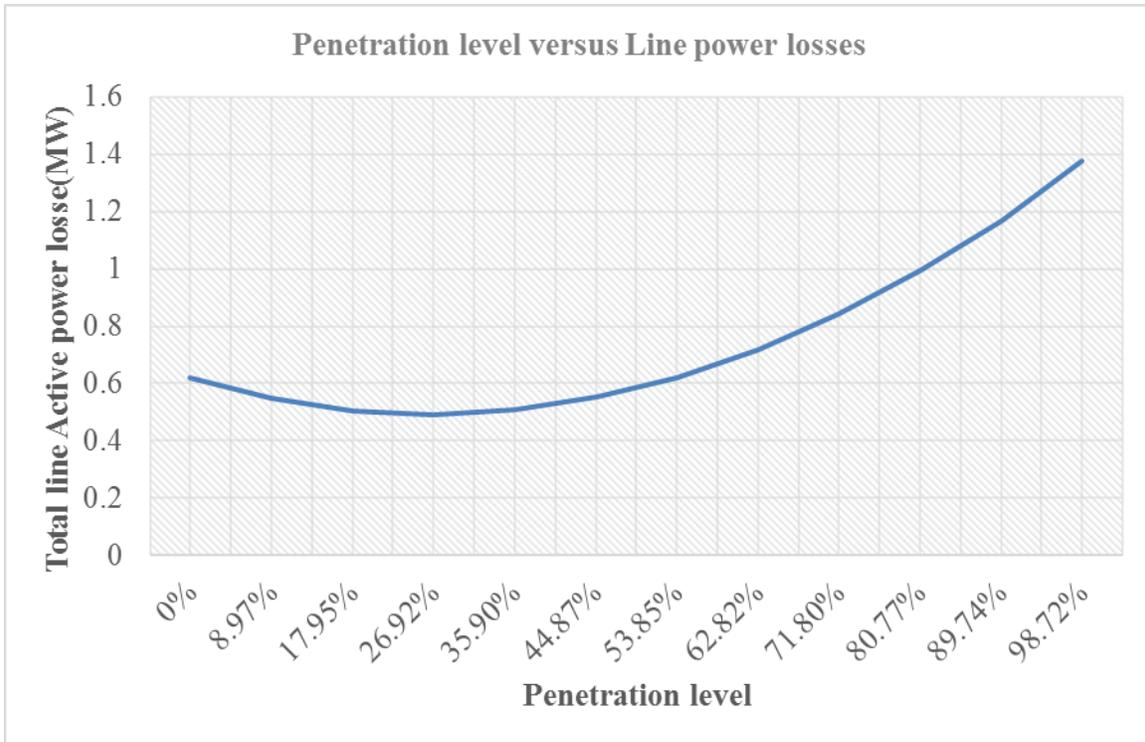
**Figure 41:** Penetration level versus Power losses at Chelstone substation
