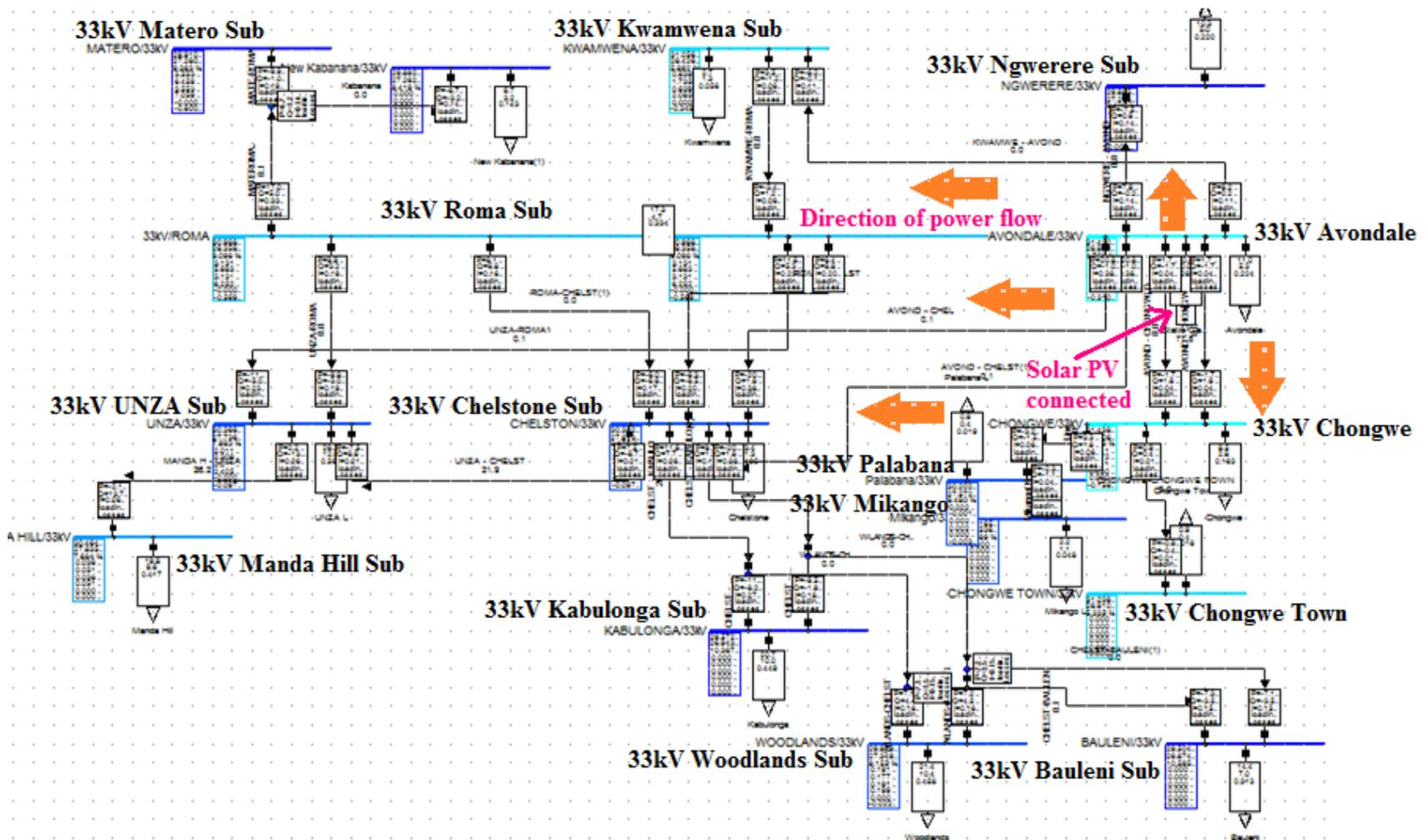
Figure 36: Overall Power flow direction change after a 90.60% (50MW) solar PV plant connection at Avondale substation
