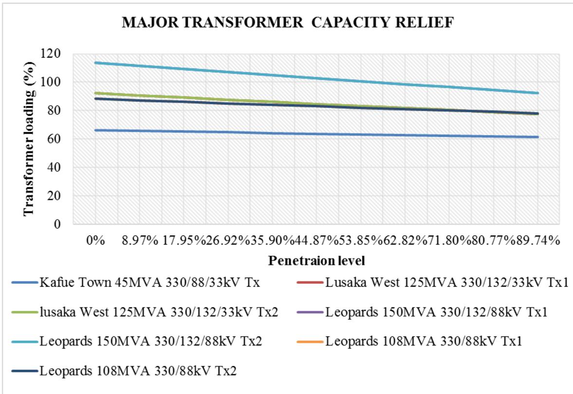
**Figure 46:** Major transformer capacity relief impact due to integration at Chelstone substation
