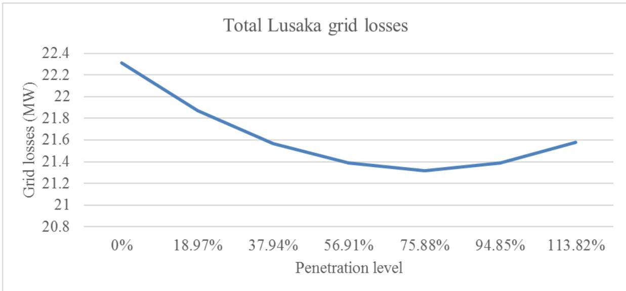
**Figure 67:** Lusaka network grid losses impact due to integration a Chilanga substation
