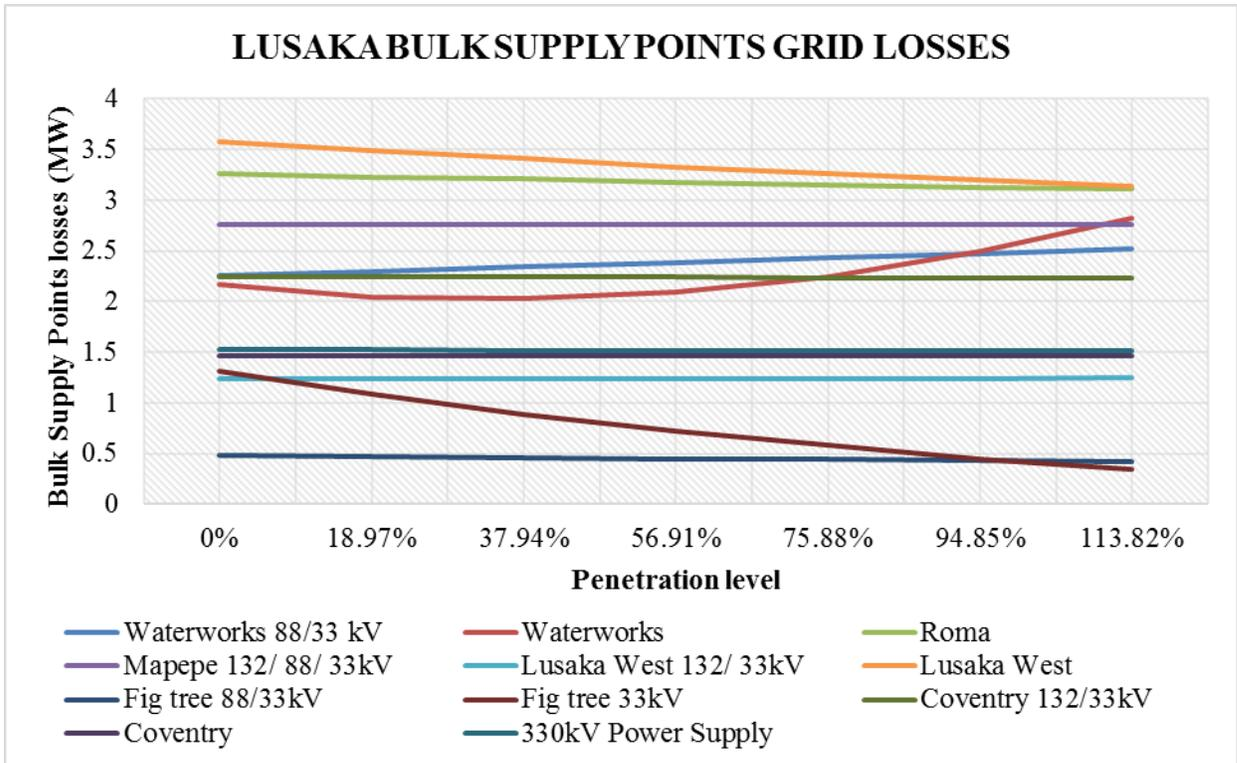
**Figure 66:** Lusaka bulk supply points grid losses impact due to integration a Chilanga substation
