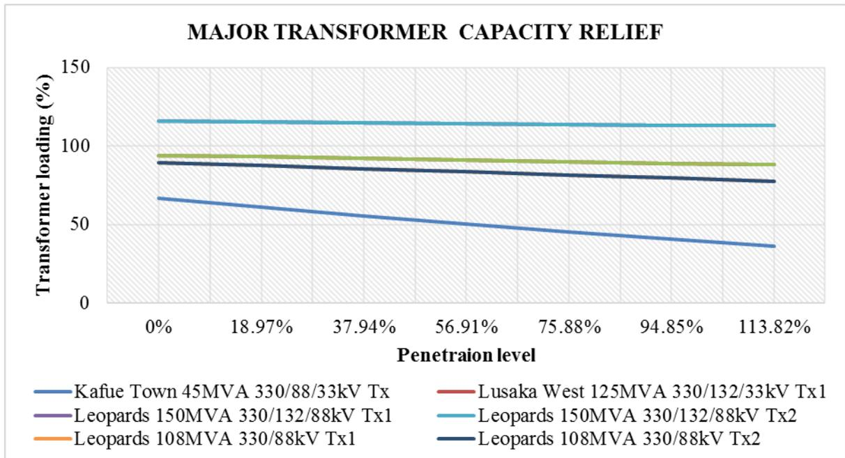
**Figure 64:** Major transformer capacity relief impact due to integration a Chilanga substation
