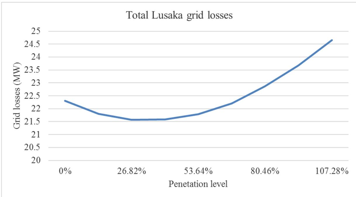
**Figure 31:** Total Lusaka network grid losses impact due to integration at Makeni substation
