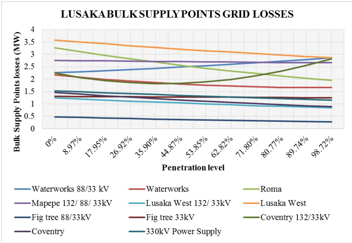
**Figure 48:** Lusaka bulk supply points grid losses impact due to integration at Chelstone substation
