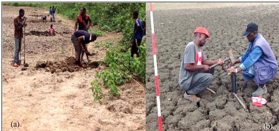
Plate 2: (a) Digging pits to determine sediment depths on the dry bed; and (b) collection of a sediment core sample from the Makoye Reservoir bed.
