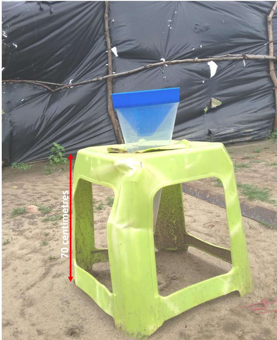
Plate 5: Onsite portable rain gauge at the Camp Site- Makoye Reservoir, Monze District, Zambia
