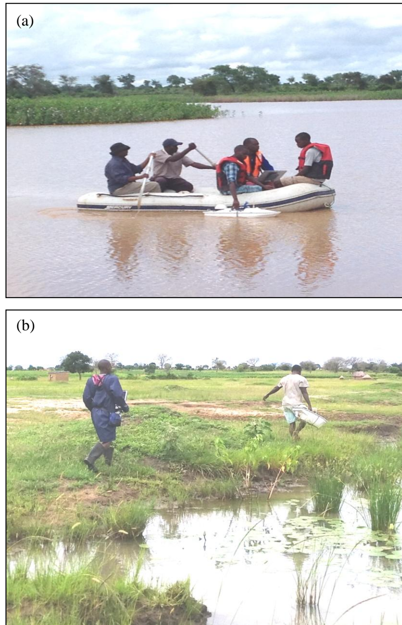
Plate 1: (a) Eco-sounding of water depth and bed morphology and (b) collecting water perimeter at Makoye Reservoir, 2017.
