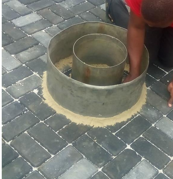
Figure 10: Installation of a double ring infiltrometer on the pavement system.
