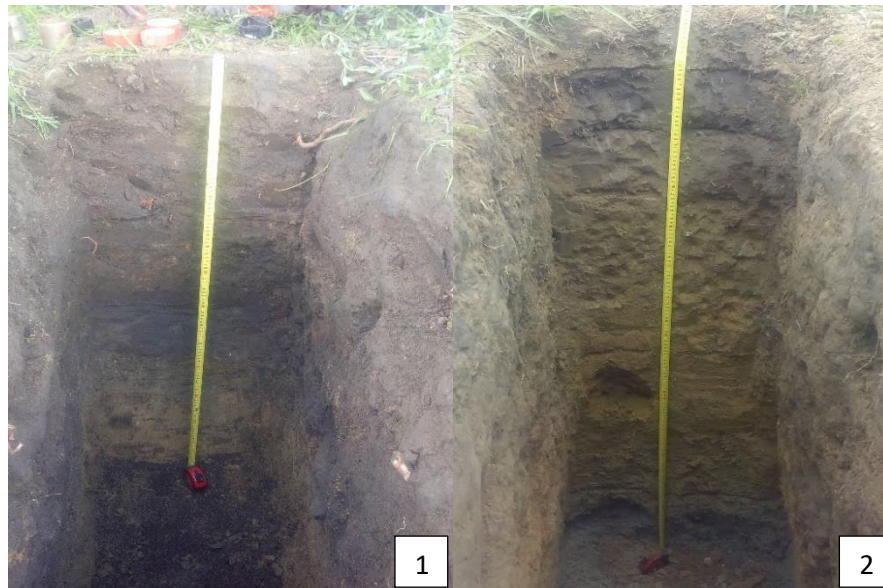
Figure 13: The central part of the urban exhibiting sufficient soil depth to support exfiltration pervious pavements.
