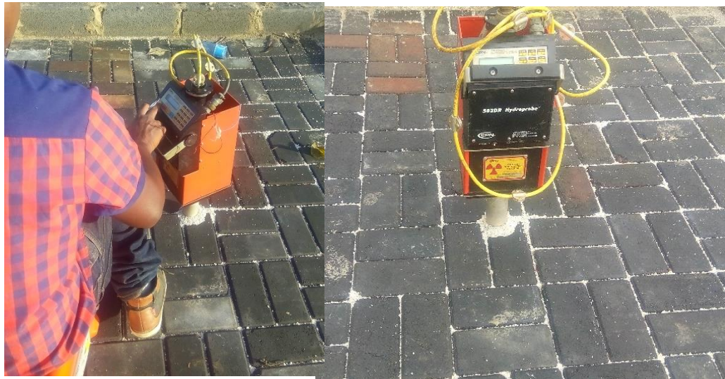
Figure 9: The gauge set to take moisture readings on the tube installed on the pavement system.
