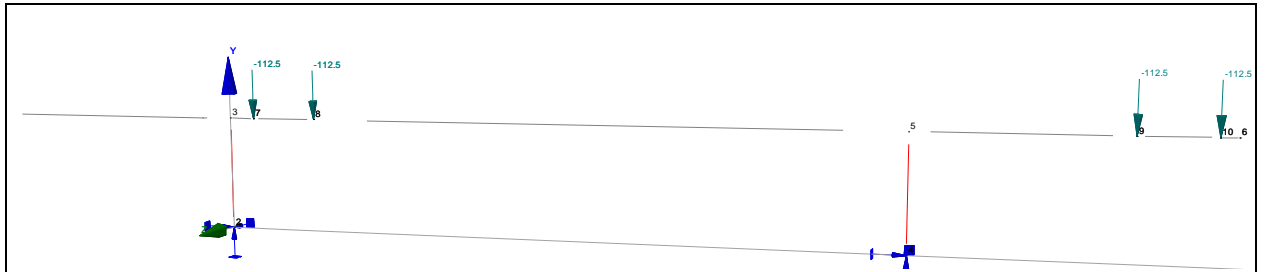
figure 4.10a:Analysis for HB vehicle with 21m axles spacing
