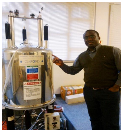
Figure 2.2: (A) A HPLC-MS assembly at H3D, UCT; (B) Prep-HPLC at H3D, UCT; (C) A 400 MHz NMR spectrometer at H3D, UCT.
