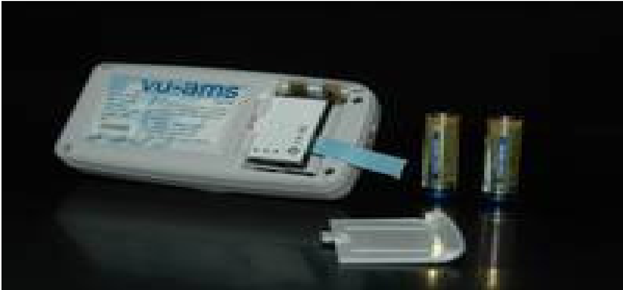
Fig.3: VU-AMS device with batteries and cover removed
