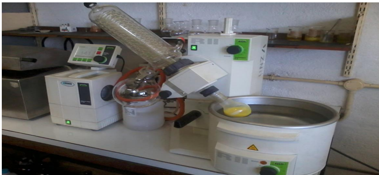
Figure 3.2: Crude extract in the drying process in a rotavapor.
