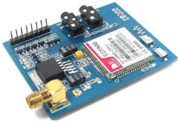
Figure 8: GSM sim900 module (by Components101, 2019)
