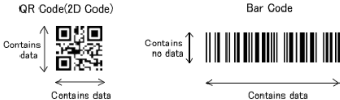
Figure 5: Comparison of QR code and Bar code (by Densowave, 2019 )
