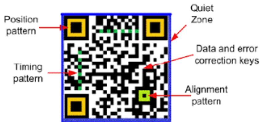
Figure 6: Elements of a QR Code (by Densowave, 2019 )
