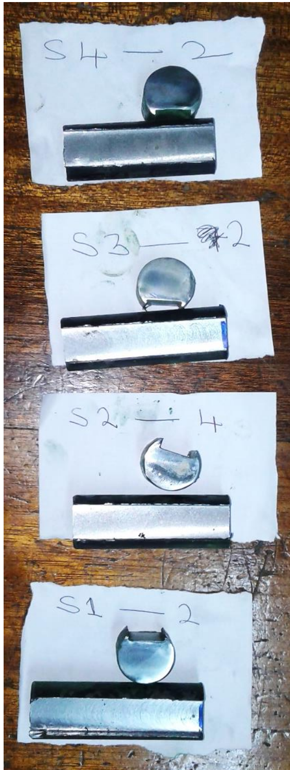
Figure 3.9. Polished and etched sections from all 4 samples
