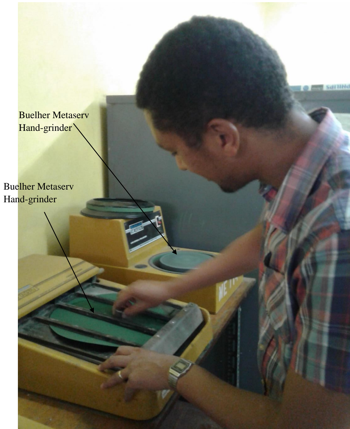
Figure 3.8. Polishing of sample workpiece section to expose the grain
