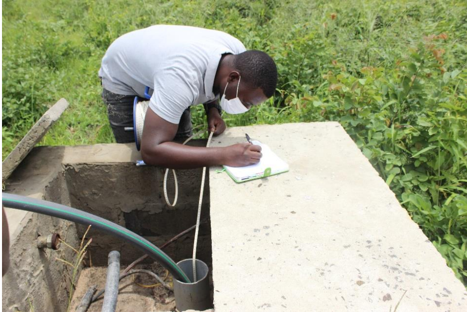
Figure 10: Measurement of the static water level in a borehole at Lukulu District Hospital, Western Zambia.
