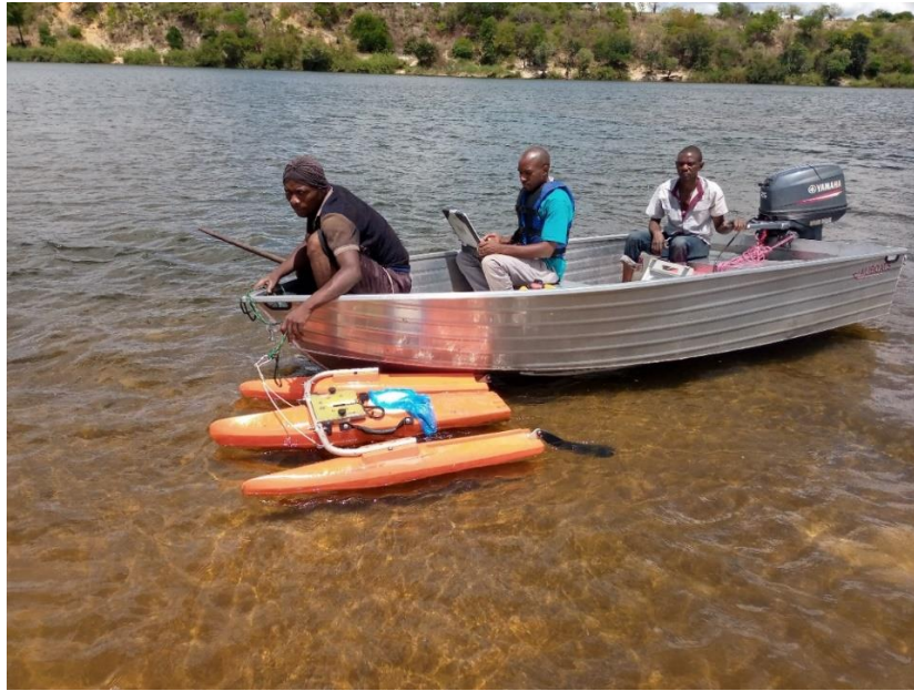
Figure 11: River discharge measurements using an ADCP equipment in Lukulu District, Western Zambia.
