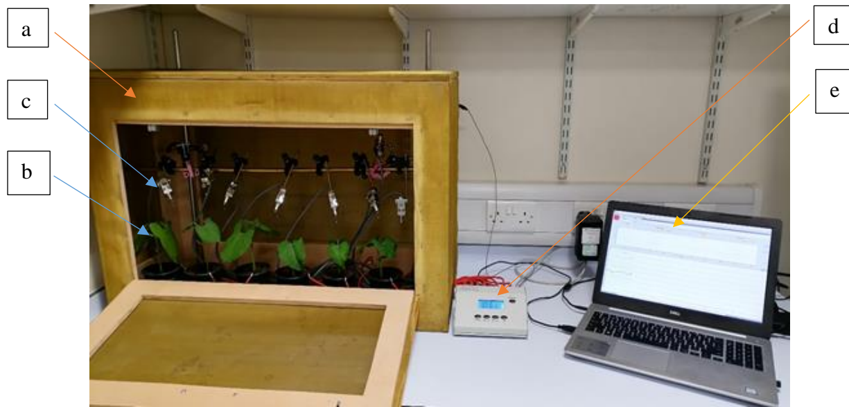
Figure 3.4: Electrical penetration graph (EPG) set-up showing the (a) faraday cage, (b) bean plants, (c) EPG probes, (d) Giga-8-EPG device and (e) a laptop computer
