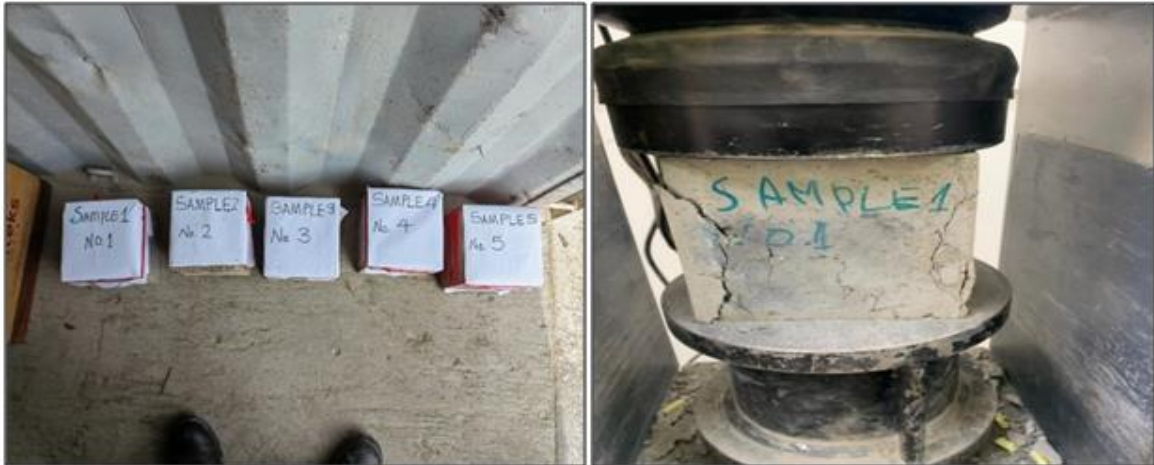
Figure 4.11: Sample preparation (a) and concrete strength testing (b)
