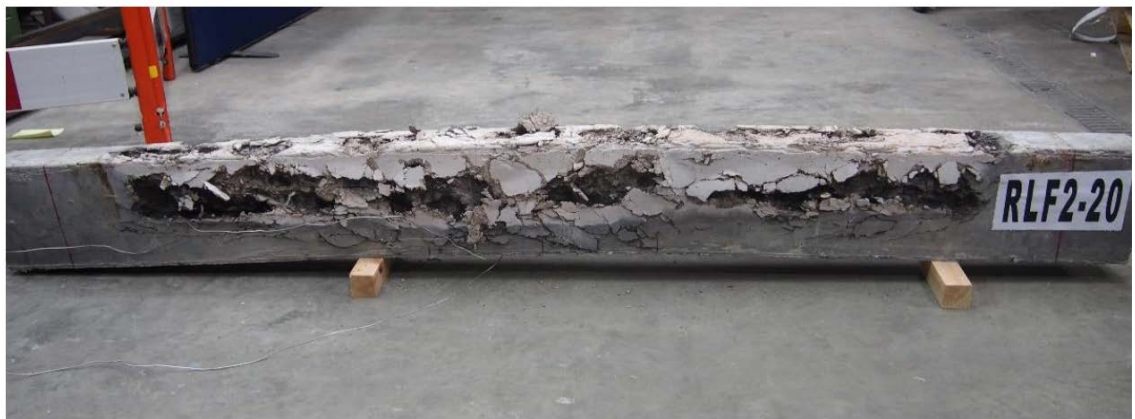
Figure 3.3: RLF2-20 beam outside the furnace after the fire test. Extracted from Kahanji (2016)
