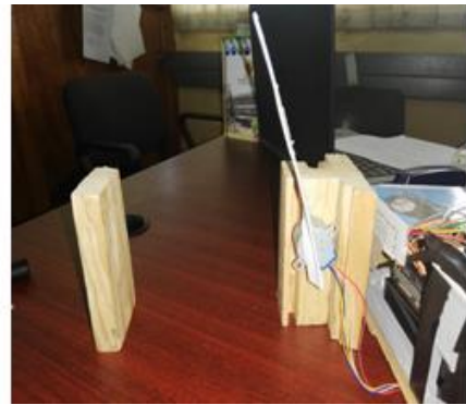
Figure 4 - 27 Gate kept open - camera capturing the number plate of every passing vehicle
