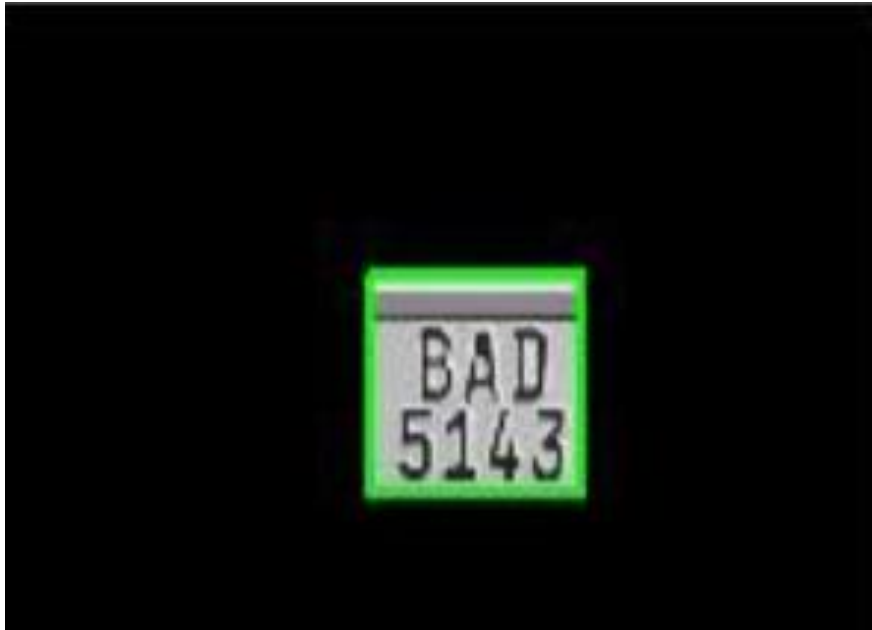
Figure 4 - 17 extracted plate region.
