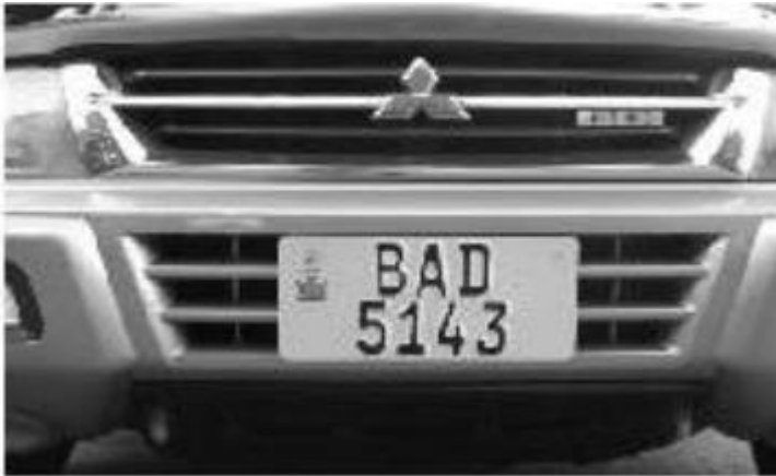
Figure 4 - 15 grey scale image dilated and eroded to remove noise
