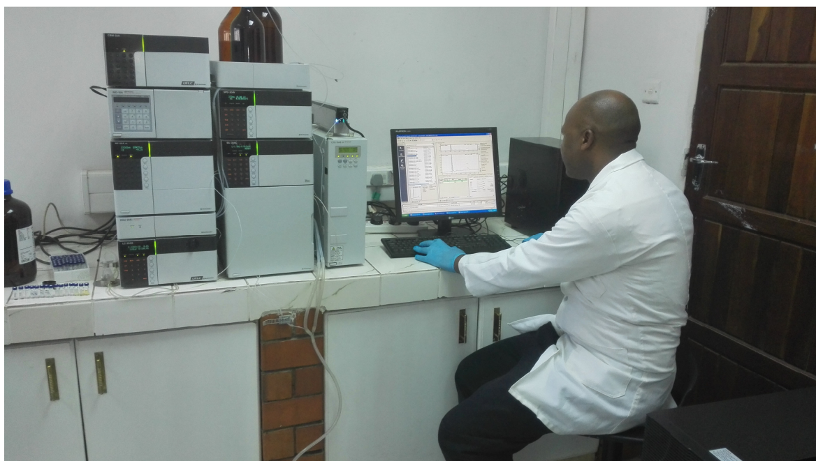
Figure 2. The HPLC and lab Solution monitor used in the analysis of the sample and generation of chromatograms.
