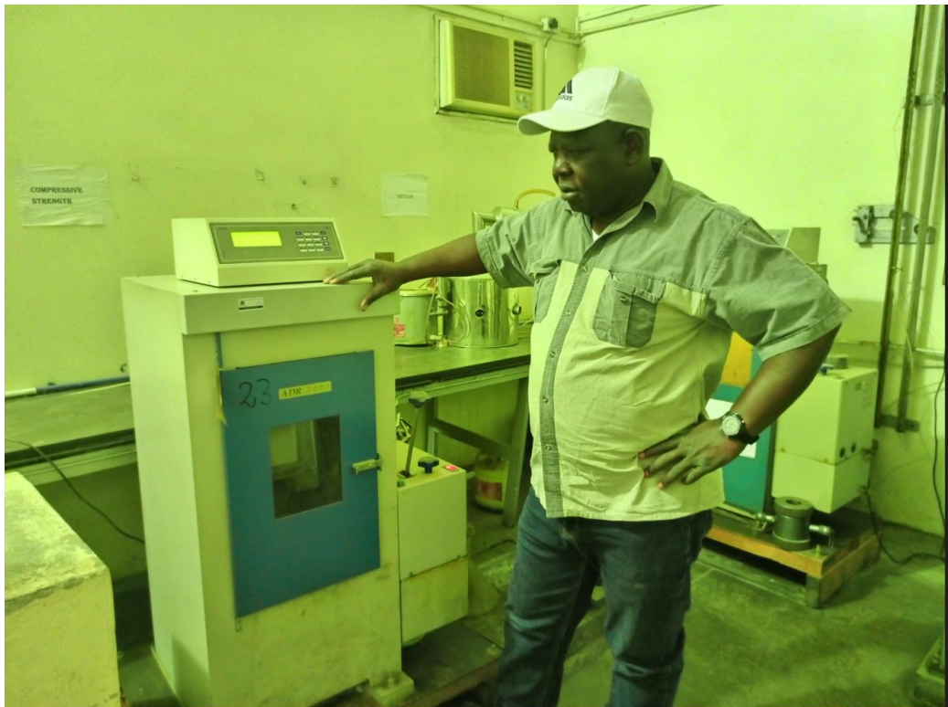
Figure 4.44: Compressive testing machine used for determining the UCS for core samples
