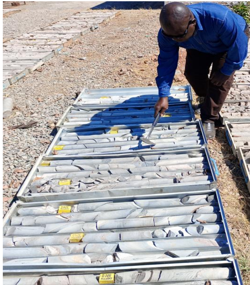
Figure 4.40: Logged BV 1171 for RQD determinations
