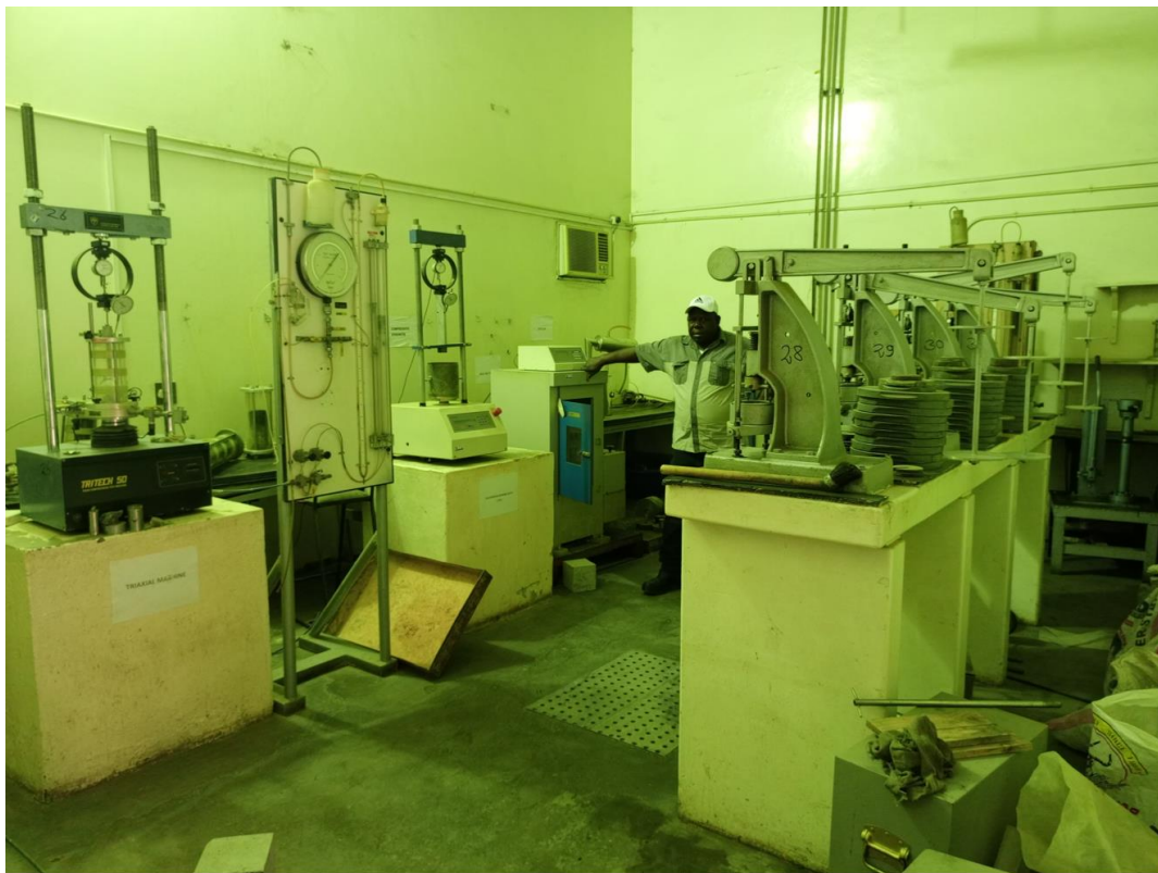
Figure 3.3: Soils and rock mechanics laboratory at Nchanga Mine of Konkola Copper Mines. The author is standing and pointing to the uniaxial compression-testing machine
