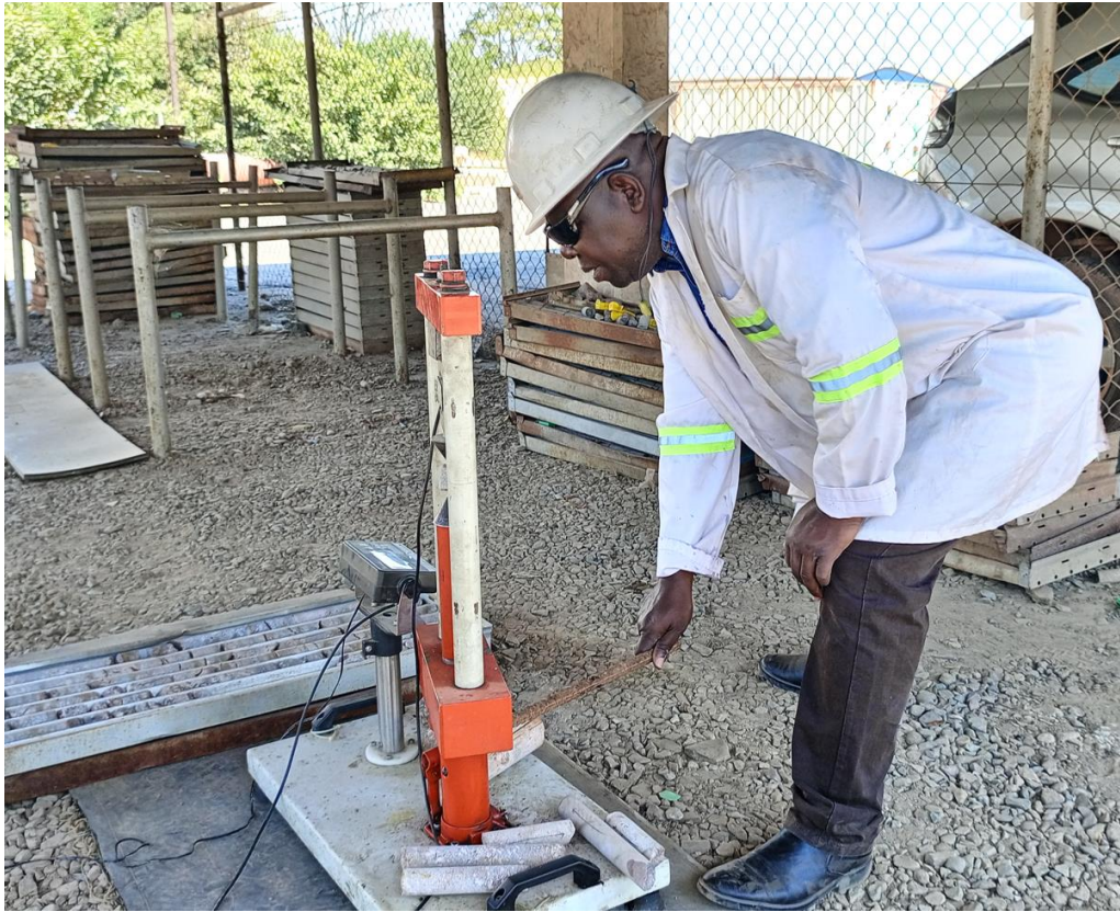
Figure 4.43: Point load testing machine used for determining the UCS for core samples
