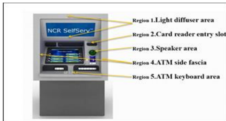
Figure 7: Skimming Device Location [Source: NCR University]
