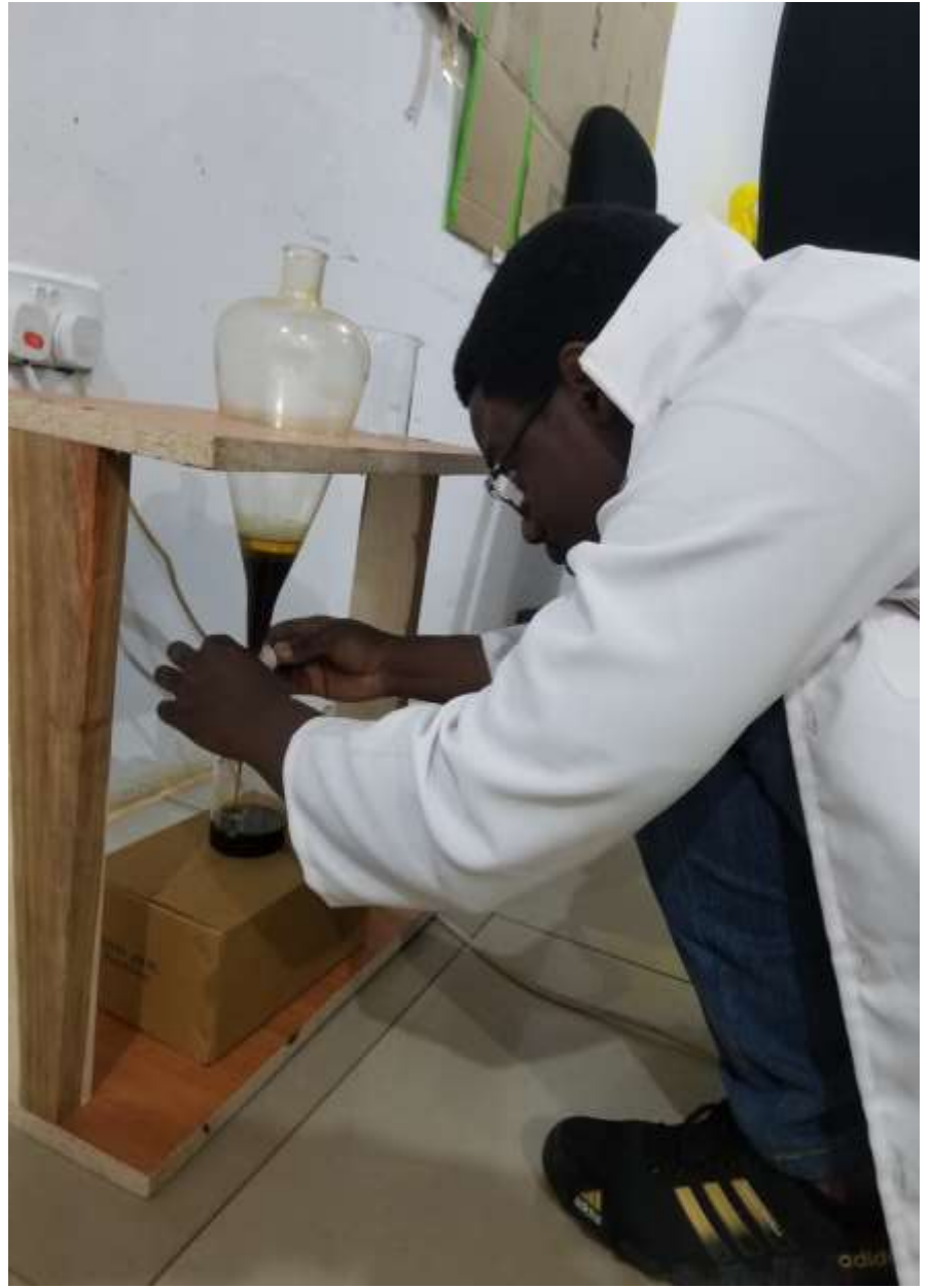
Figure 3.3: Tobacco extract stored in a glass tube (A); separating funnel used to drain off waste of tobacco extract (B).
