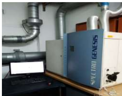
Figure 8: Inductively Coupled Plasma-Optical Emission Spectrometer. Photo captured from the University of Witwatersrand Analytical Laboratory, Johannesburg, South Africa
