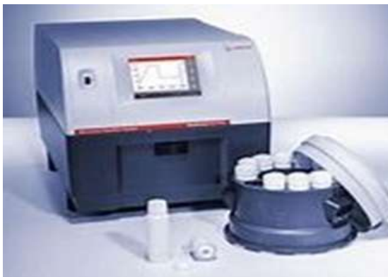
Figure 7: Anton Paar Microwave Go Digester. Photo captured from the University of Witwatersrand Analytical Laboratory, Johannesburg, South Africa
