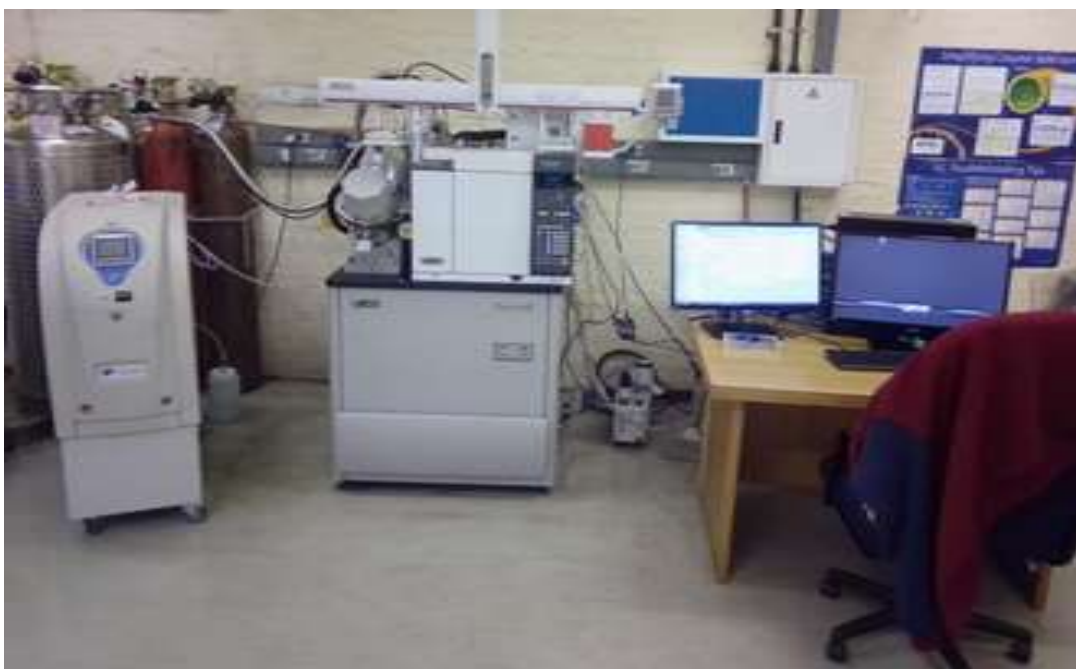
Figure 6: Gas Chromatography x Gas Chromatography/Time of Flight Mass Spectrometer. Photo captured from the University of Witwatersrand Analytical Laboratory, Johannesburg, South Africa
