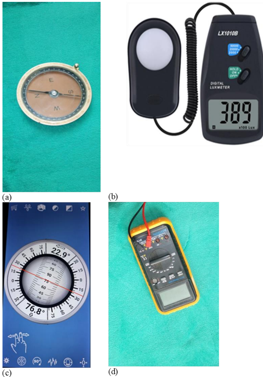
Figure 7: A picture of magnetometer (a), luxmeter (b), inclinometer (c) and, multimeter (d) All angles of orientation were measured with reference to the North direction as illustrated in Figure 8. A multimeter was used for voltage and current measurements. See appendix 11 for the raw data
