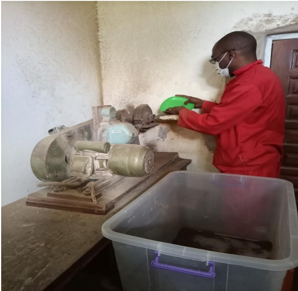
Figure 4: Grinding of Black soldier fly larvae into a meal
