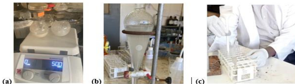
Figure 30: (a) Magnetic stirring (b) Washing (b) Column chromatography.
