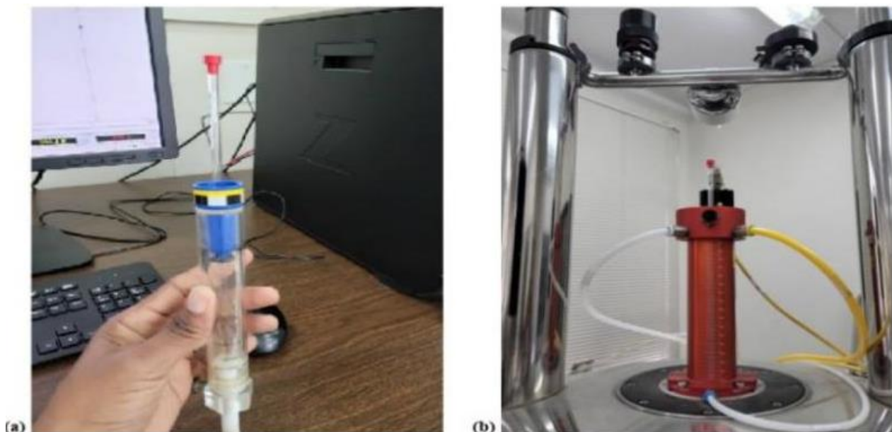
Figure 34: (a) Sample dissolution in \text{DMSO-}d_6 (b) Sample tube insertion into spinner.
