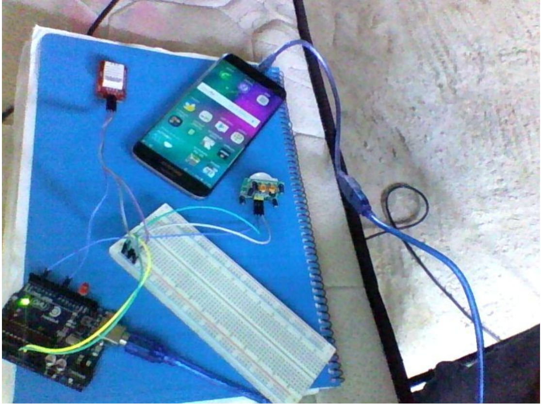
Figure 31- Early version of sensor node with mobile phone for network connectivity
