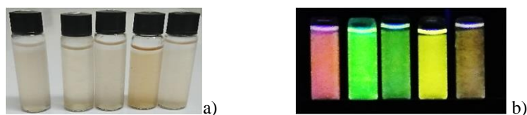
Figure B.1: CdSe-QDs solutions in, from left to right, synthesised using 0.00 M, 3.21 \times 10^{-5} M, 6.42 \times 10^{-5} M, 9.63 \times 10^{-5} M and 1.28 \times 10^{-4} M of PVA a) in ordinary light and b) under UV-light at 366 nm.
