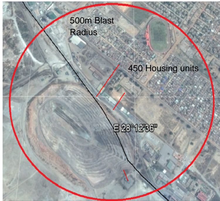
Figure 31: A total of 450 Housing units within 500m safe blast radius (Satellite image)
