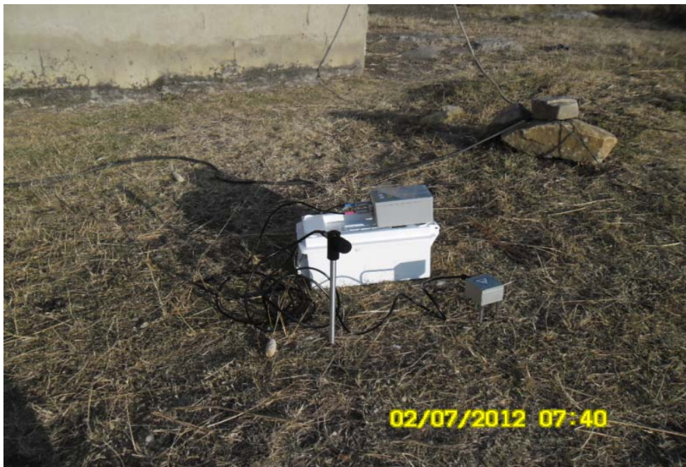
Figure 33: NOMIS seismograph mounted on the ground
