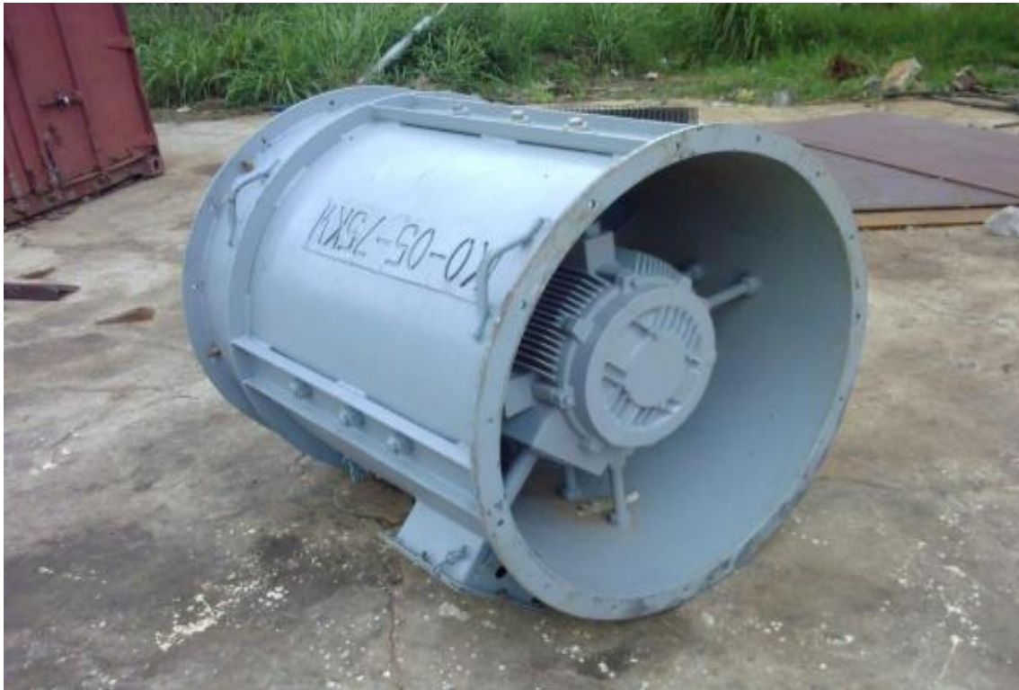
Figure 24: An Underground booster fan
