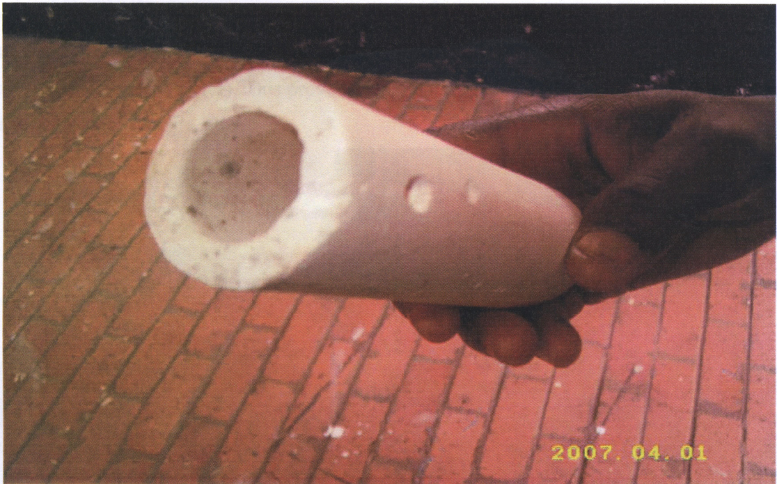
Plate 19: Ceramic water filter candle produced by NISIR
