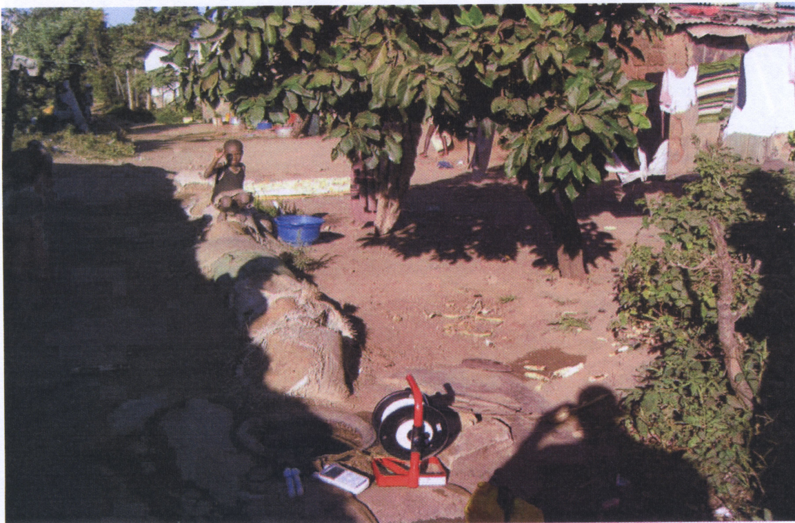
Plate 6: Well Number 2 (Mr. Aibaki Lungu's well) with sandbags used as protection against running water. Some of the equipment used during the study for in situ analysis Left to right- Multifunction Horiba meter and Water level Meter (on a reel)
