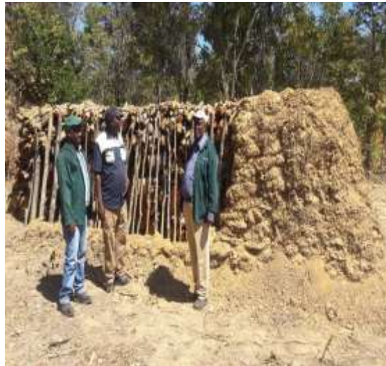
Figure 3.2: Traditional charcoal kiln covered with earth (Field photos)
