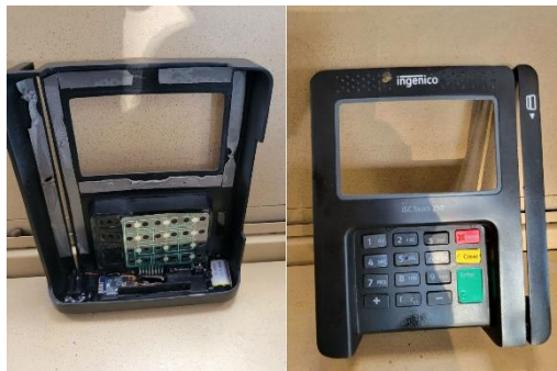
Figure 2 POS machine card skimmer/cloner [9]
