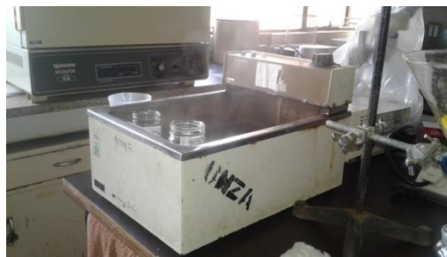
Figure 3.10: Vaporization of Solvents in water bath at 105°C
