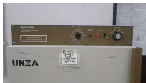
Figure 3.5: Yamato Drying oven pre-set at 35°C
