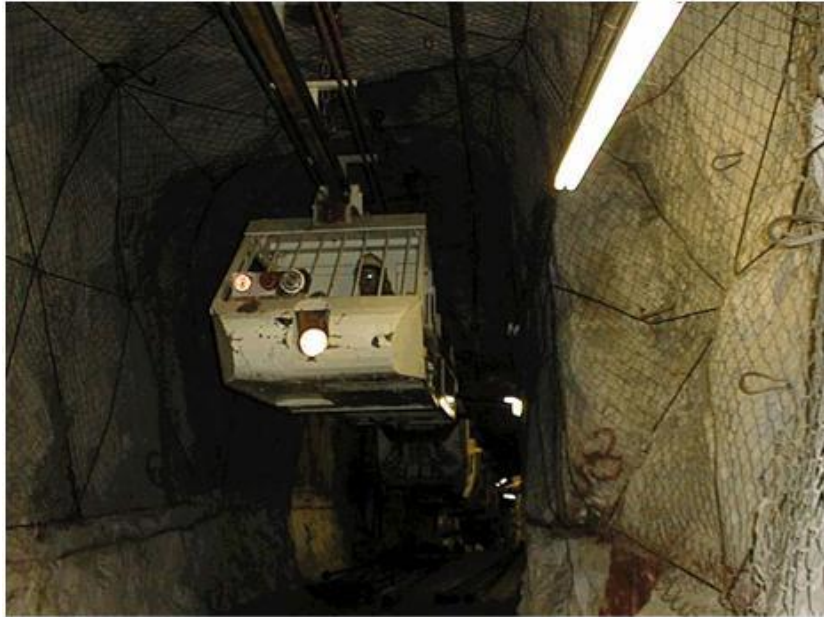
Figure 6.1: Decline support system for monorail installation (Scharf, 2007)
