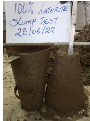
Figure 4.14: Slump test for 100% LCA fresh concrete
