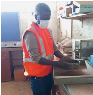
Figure 4.2: Sieving of crushed LCA using 0.425mm sieve
