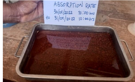
Figure 4.13: LCA absorption rate test
