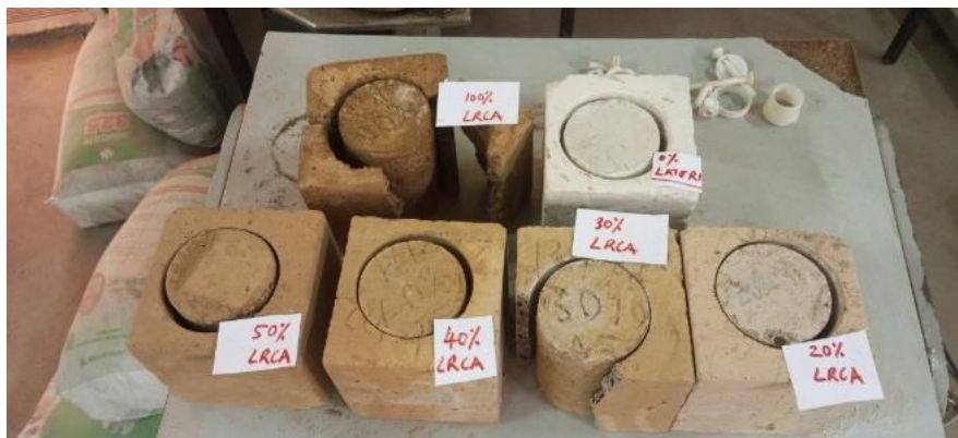
Figure 4.50: Achieved cores from the cube specimens
