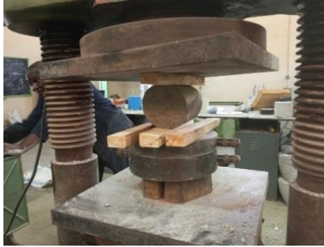
Figure 4.36: Split testing of a cylindrical specimen
