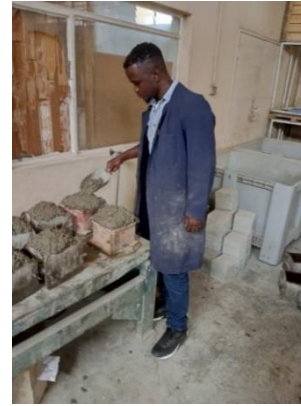
Figure 4.15: Vibrating of fresh Concrete in moulds
