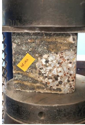
Figure 4.45: Example of Spalling and pitting on the 40% Specimen
