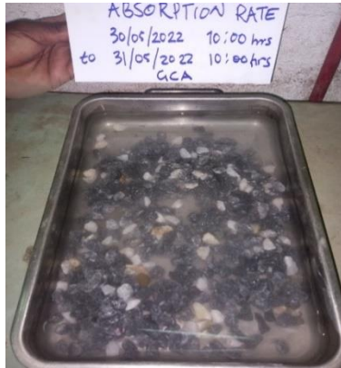
Figure 4.12:GCA Absorption rate test
