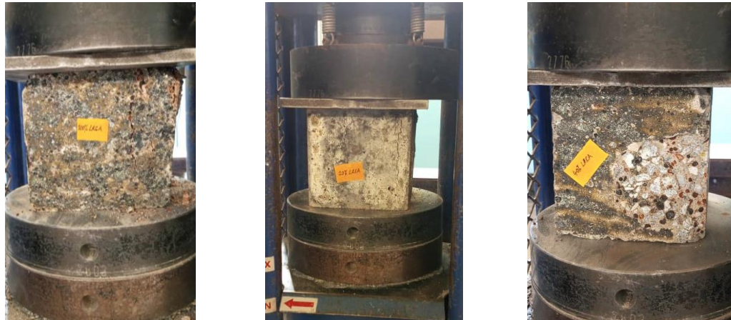
Figure 4.40 : Compressive Strength Testing of cube specimens after exposure to high temperature
