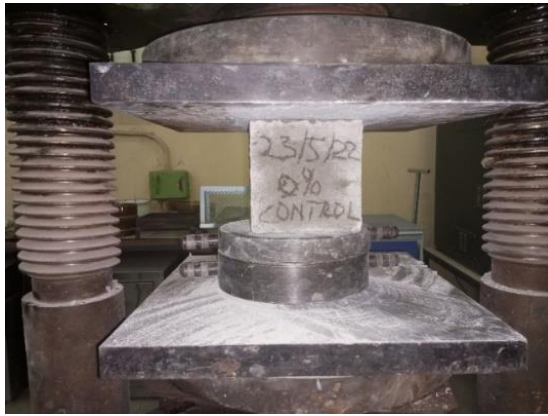
Figure 4.25: Compressive Strength Testing
