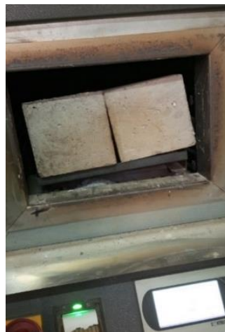
Figure 4.39: Concrete Cubes in electric furnace after exposure to elevated temperature
