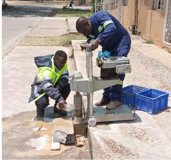
Figure 4.49: Coring through concrete cubes to obtain specimens for absorption and sorptivity tests of concrete
