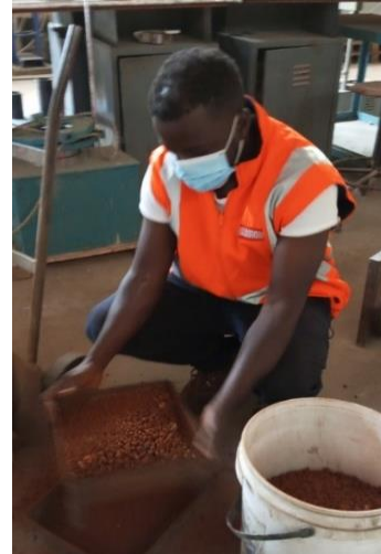
Figure 4.8: Screening of Laterite using Sieve No. 4
