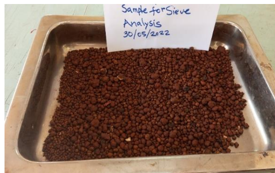
Figure 4.9: Washed LCA sample for sieve analysis
