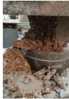
Figure 4.26: Failure mode for the 100% LCA Cubes at 7 Days
