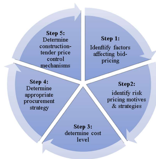
Fig. 13.2: Construction price negotiation process (By the author based on a literature review and research findings; Paek & Lee, 1993; Gudienè, et al., 2013)
