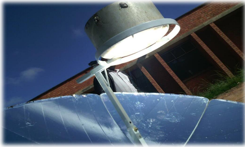
Figure 3.4: Heat energy focussed onto a pot.
