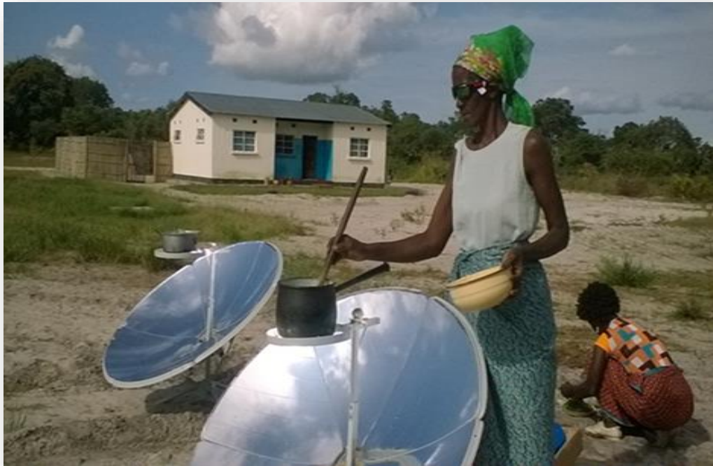
Figure 3.5: Women cooking on solar cookers (on a partially cloudy day) in Western province
