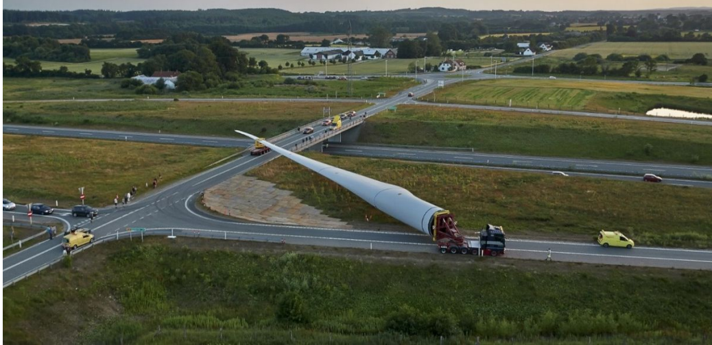
Figure 17: Transportation of an 83.5 m long WT Blade from Danish SSP Technology ( SSP-Technology, 2017 )
