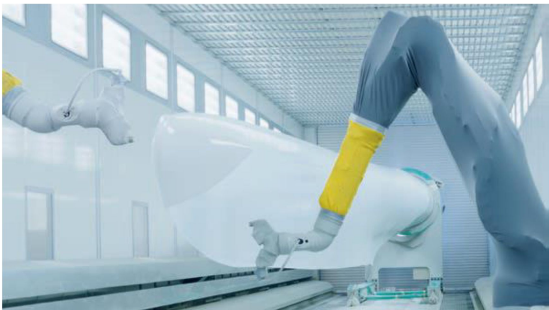
Figure 11: Painting Robots for WT blades ( Sainz, 2015 )
