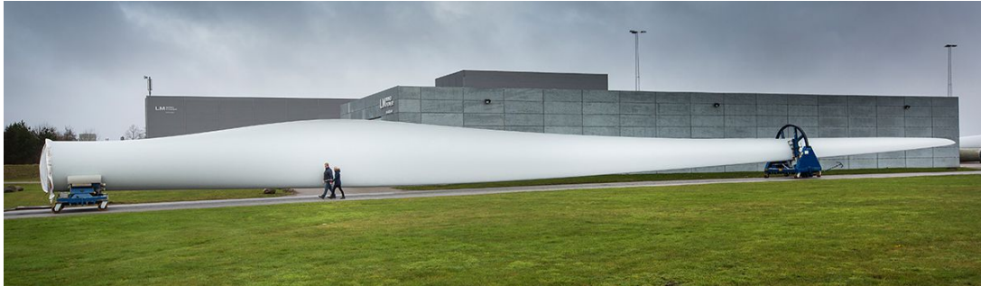
Figure 12: A Finished LM Blade Ready for Shipping ( LM Wind Power, n.d. )
