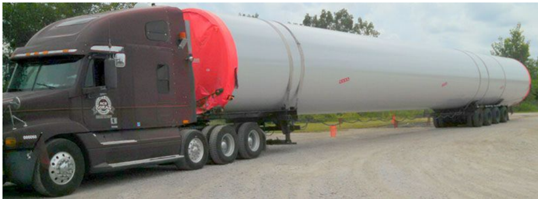
Figure 18: Transportation of a WT Tower Section by Ace Doran Haulage and Rigging ( Ace-Doran, 2017 )
