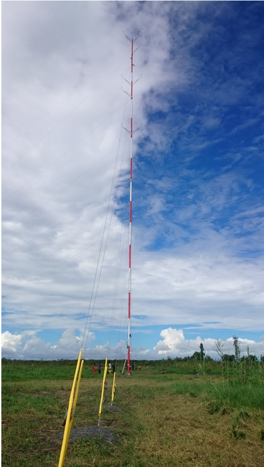
Figure 5: The NRG 60 m Mast Installed at Kasomalunga in Luapula.
