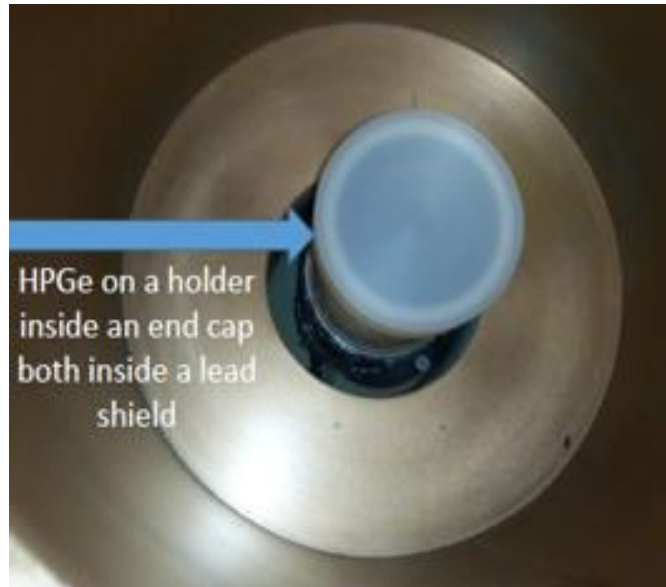
Figure 9: Inside the lead Shield showing detector holder and end cap
