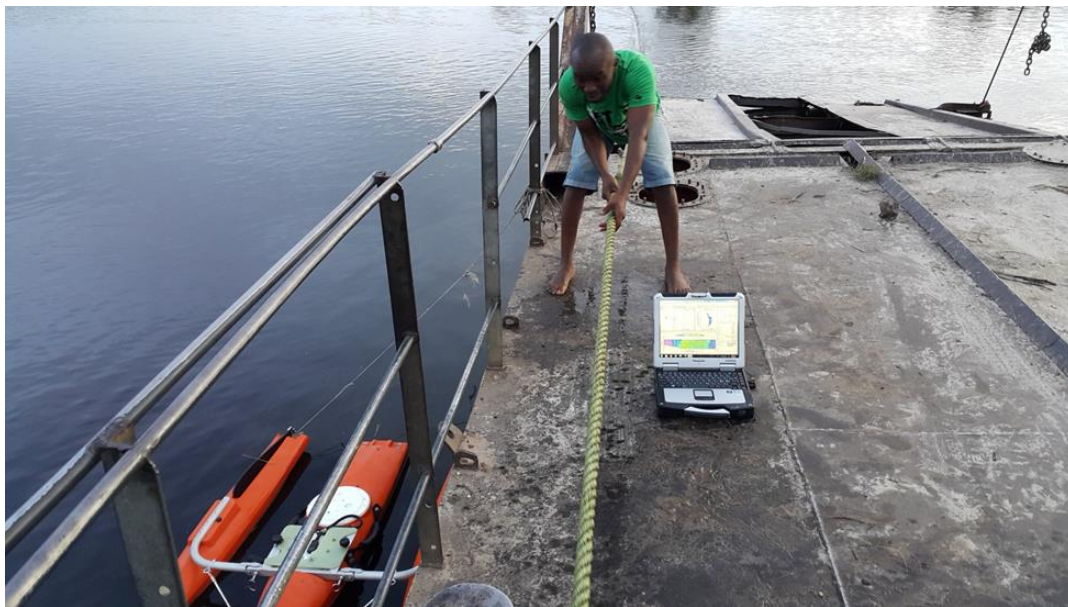
Figure 3.7: Method used in measuring discharge at Kalabo Hydrometric Station using a tagline tied end to end with the ADCP tied to the boat, Barotse Floodplain, Western Zambia A tough-book computer communicated with the ADCP via Bluetooth settings. This made the reading easier and convenient unlike the serial connections that required cables. The software programme used in the communication between the tough-book and the ADCP is called Broad
