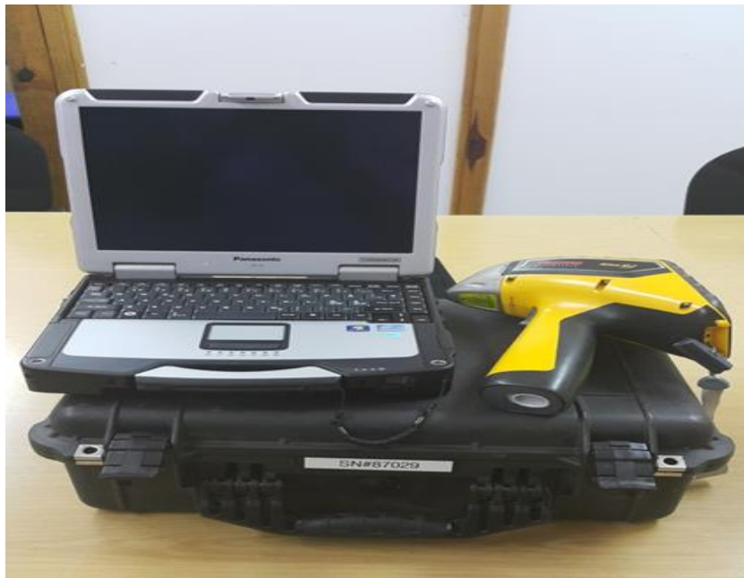
Figure 3.10: XRF, case and tough book computer where the NDTr software was installed for downloading readings, used for measurements on the Barotse Floodplain, Western Zambia
