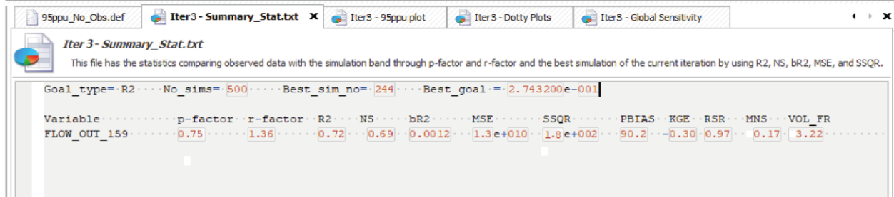
Figure 4.24: Summary statistics comparing observed data with the simulation band through P-factor and R-factor and the best simulation of the current iteration by using Coefficient of Determination ( R^2 ), Nash Sutcliffe (NS), Modified Coefficient of Determination ( bR^2 ), Mean Square Error (MSE), Sum of Square Residual (SSQR), Percent Bias (PBIAS), Kling-Gupta Efficiency (KGE), Root Mean Square Error (RSR), and the Overall Water Balance Fraction (VOL_FR). This was for the three iterations (a), (b) and (c)
