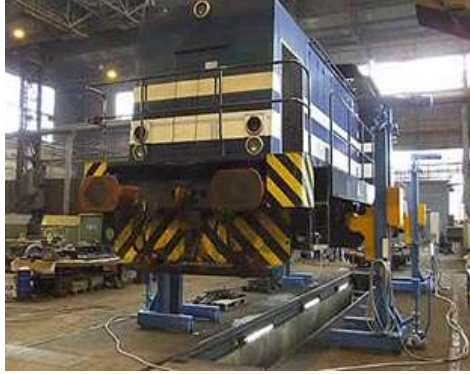
Figure 3.6: DE locomotive suspended on lifting jacks
