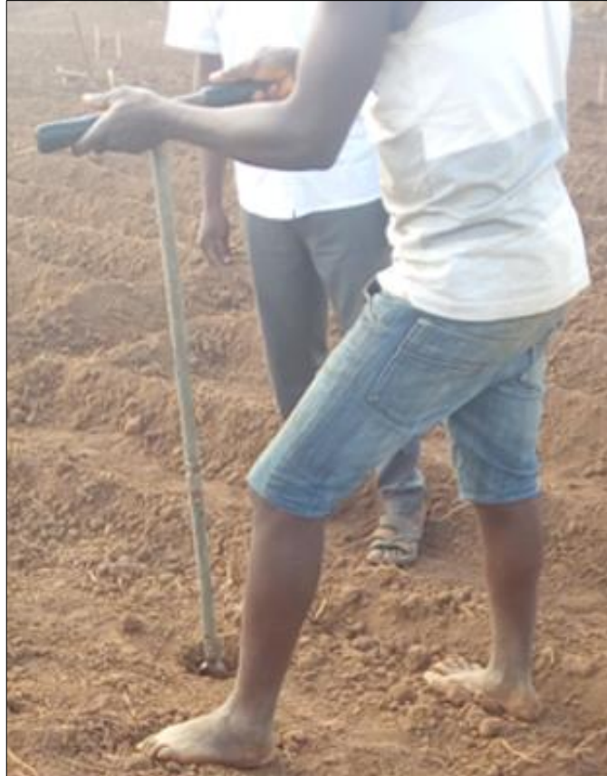
Figure A1.2: A hand auger is used to get soil samples from different treatment plots
