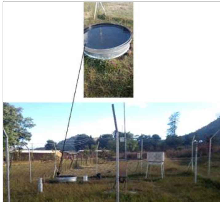
Figure 3.11: Meteorological local weather station in Dedza-Malawi having Class A Pan
