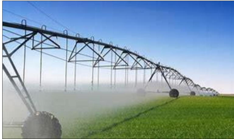
Figure 2.6: Center pivot irrigation system (Source: Yan et al. , 2021)
