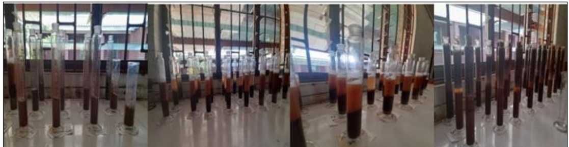
Figure A1.5: Determination of soil texture in Kasinthula Research Station Lab
