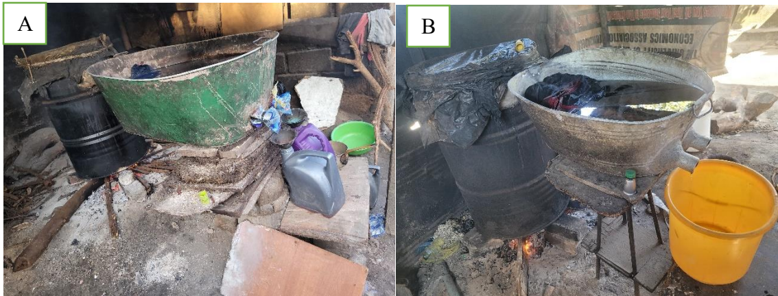
Figure 4.10: A. Water sachets funnels. B. No funnel to direct distillate and collection in a bucket.
