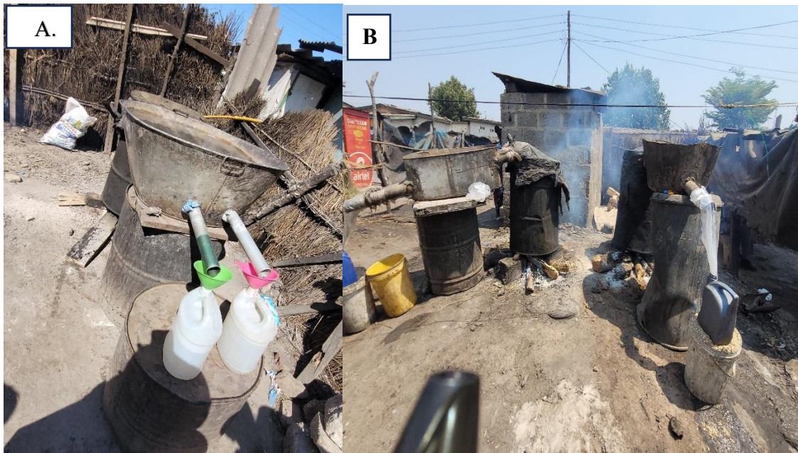
Figure 4.4: Distillation units: A. is double barrel, and B. is single barrel condenser.
