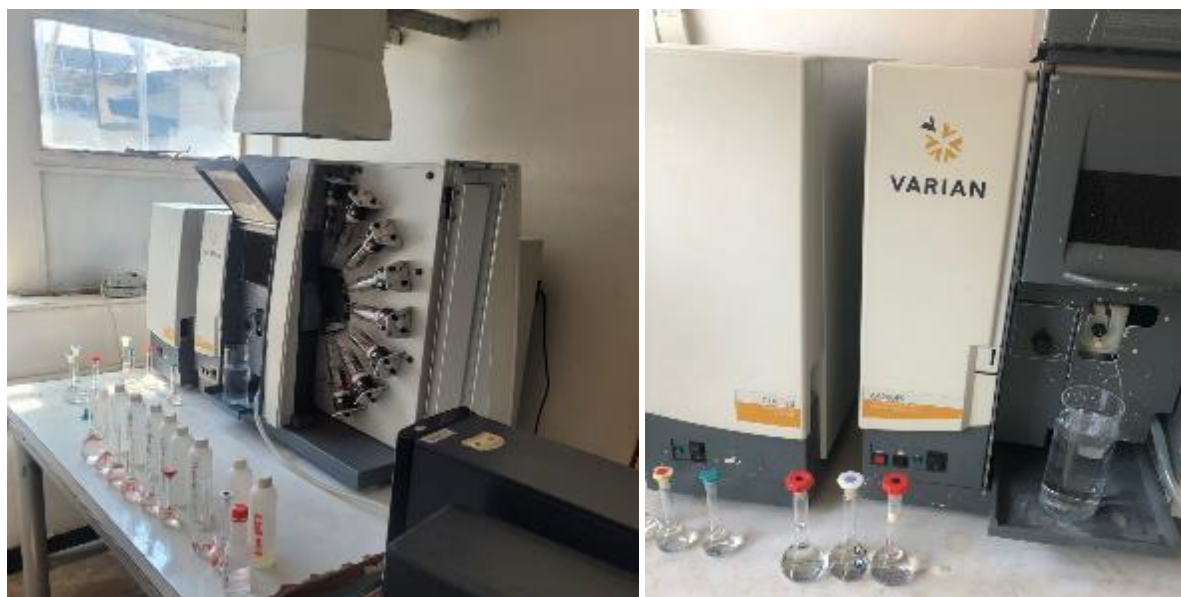
Figure 3.6: Varian AA280FS AAS used to determine the Fe, Cu and Cd content.
