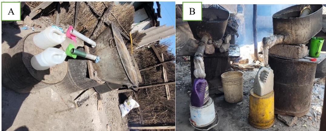
Figure 4.9: A. Double barrel condenser and B. Single barrel condenser.
