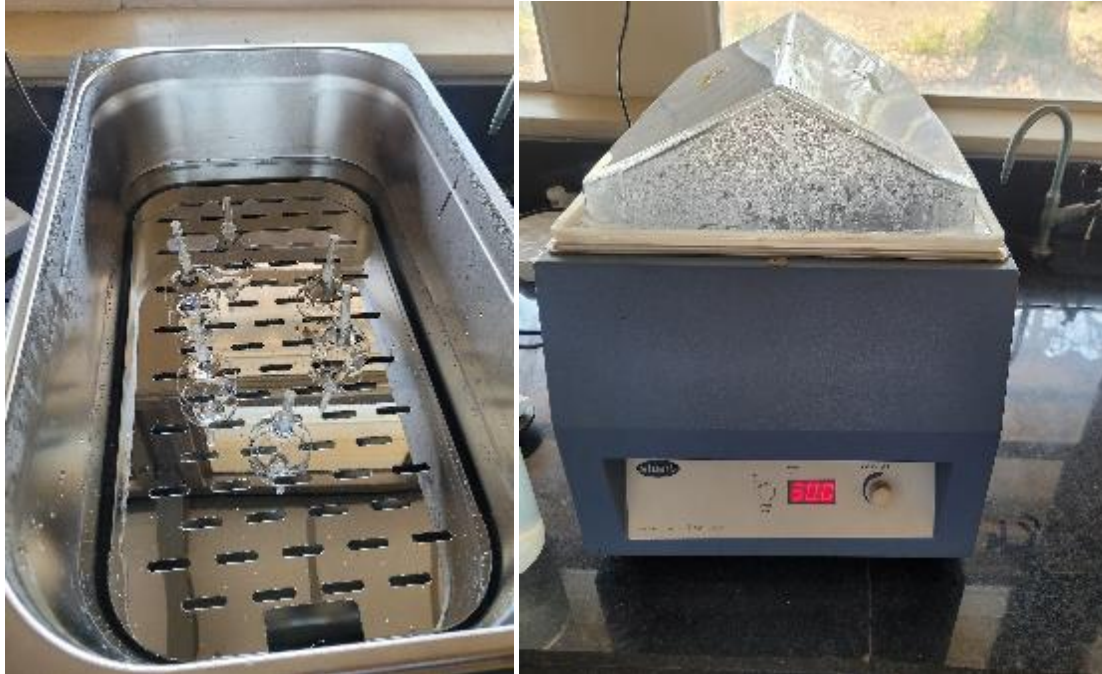
Figure 3.3: Attemperation of distillate samples to 30°C in a Stuart water bath.
