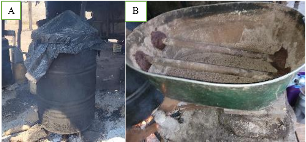
Figure 4.8: A. Distillation drum covered by a black polyethene sheet and secured with a rubber rope; B illustrates the condenser.
