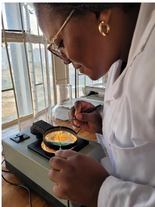
Figure 3.8: Counting of colonies on plates using a Fisher accu-lite colony counter.
