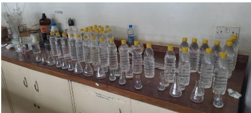
Figure 3.2: Sample preparation for titration to determine total acidity.
