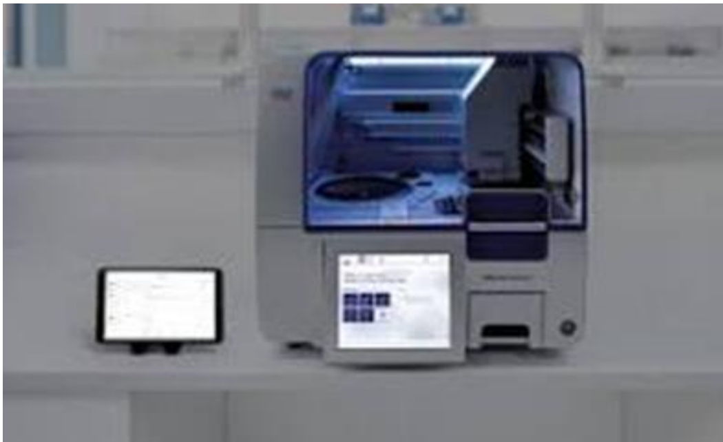
Figure 3.2 Qiacube Connect automated device used for DNA extraction in various forensic samples such as buccal swabs, bone tissue, blood, saliva, vaginal swabs etc. https://www.qiagen.com (21/05/2025).
