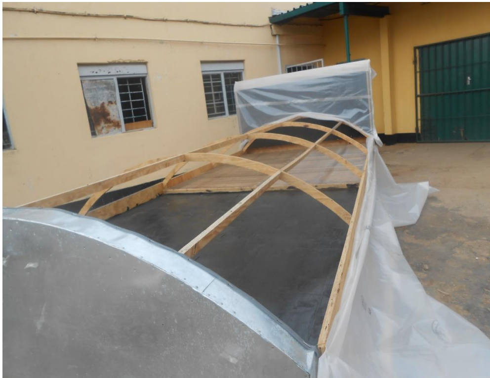
Figure 3.4: The open dryer showing the solar absorber painted black and the drying tray.
