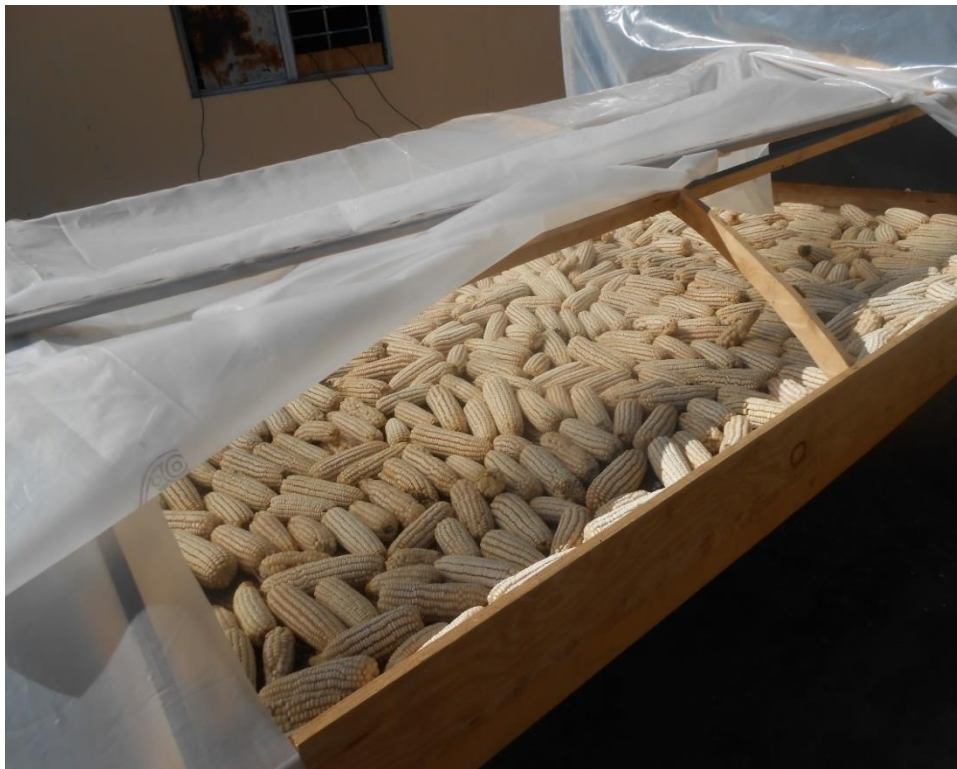
Figure 4.9: Maize being dried in the solar tunnel dryer (STD).
