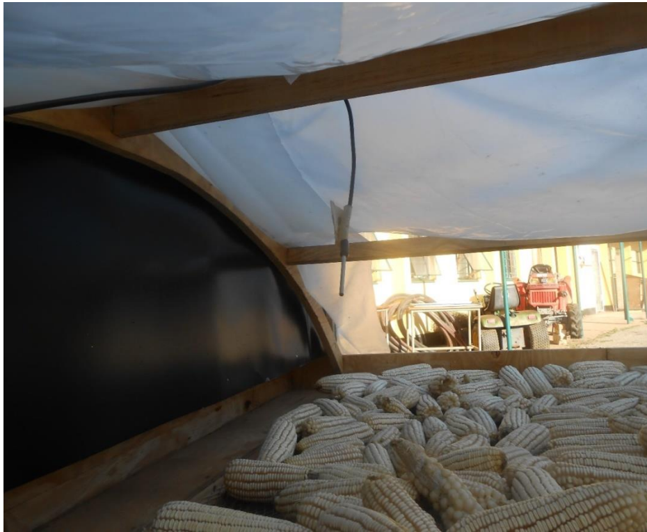
Figure 4.6: Pictorial view of probe measuring air temperature at dryer exit.
