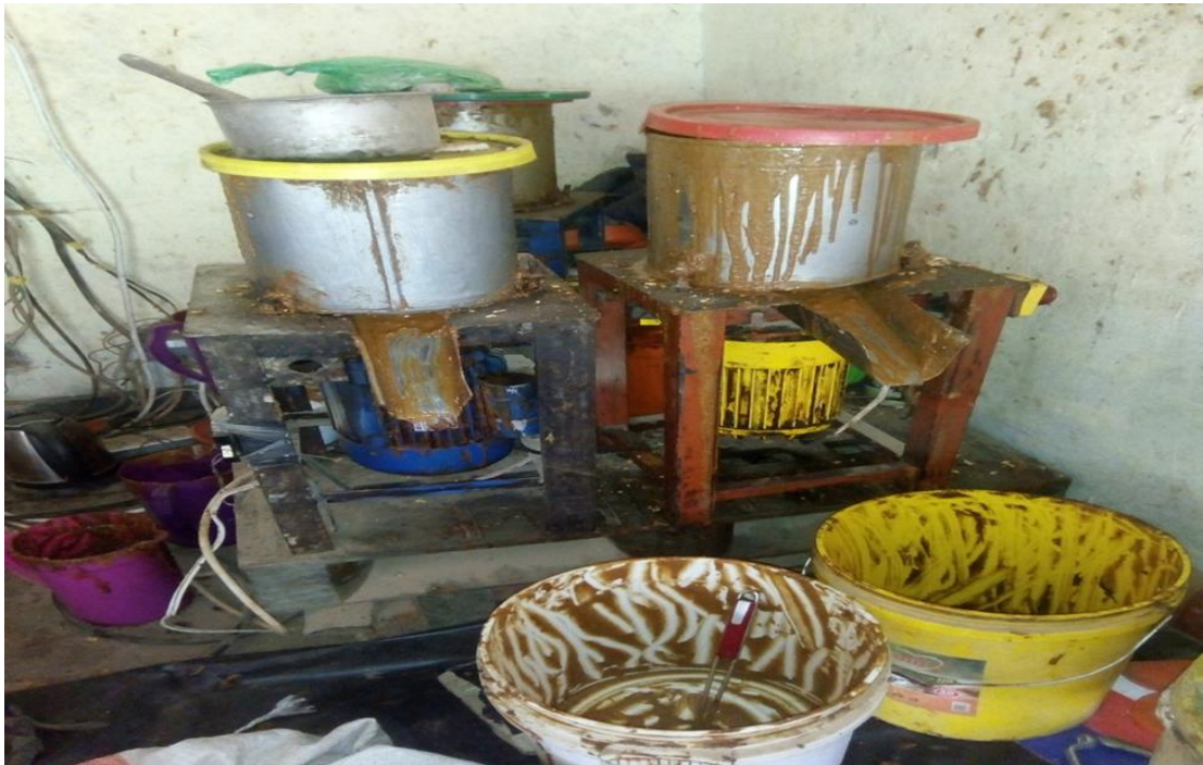
Figure 5. 6: Machine used by local traders to process peanut butter. (Source: Field data, 2018)
