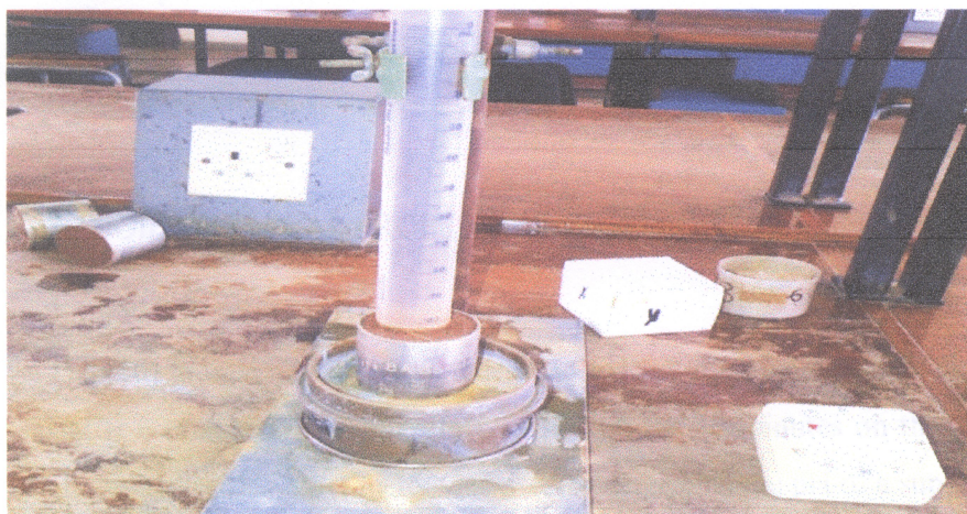
Figure 1: A laboratory Setup used to determine infiltration rate in undisturbed soil samples
