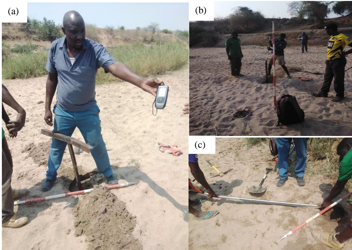
Figure 10: Sediment Coring (a) and (b); Using angle bars (c) Measuring sediment depth.
