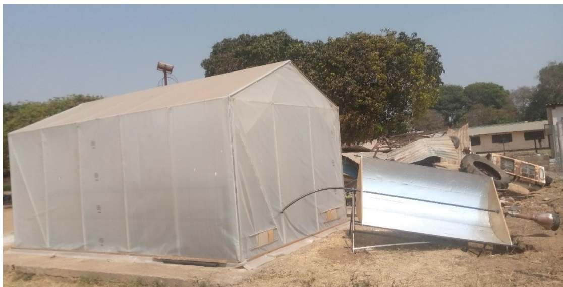
Figure 3. 13 Experimental setup of GSD connected with PTSC before noon
