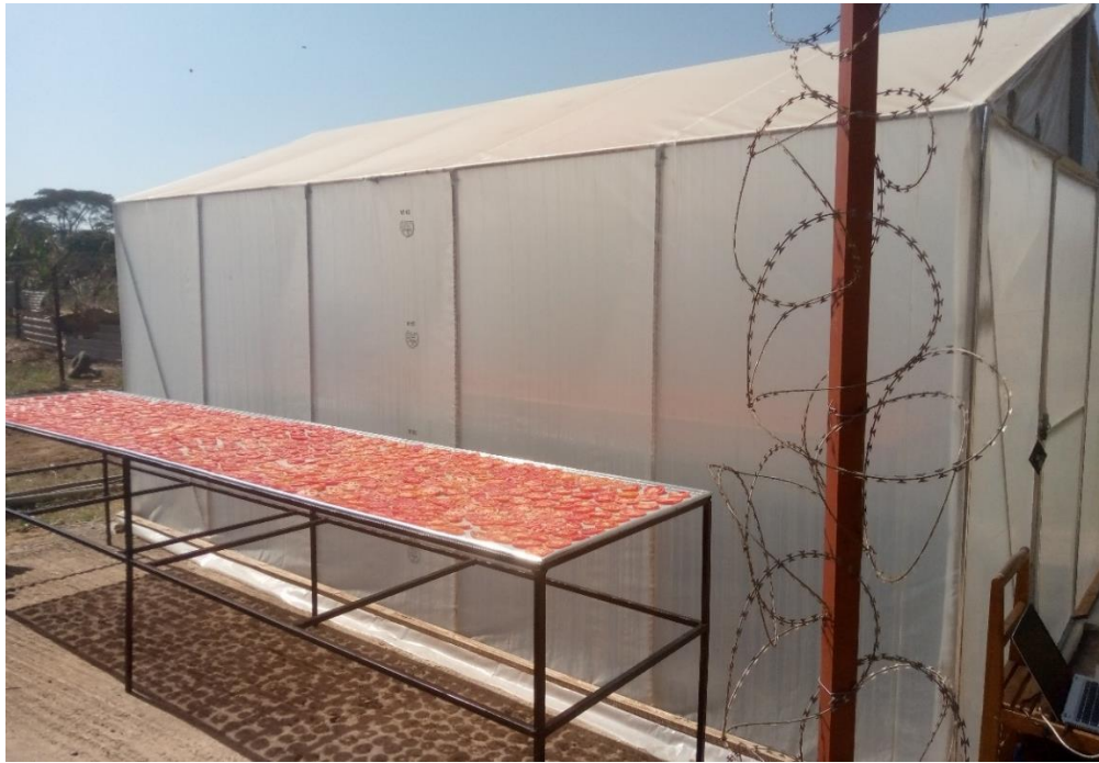
Figure 3. 11 Load test of the GSD with tomatoes with equal amounts being dried using OSD method (tray positioned outside the GSD under the open sun).
