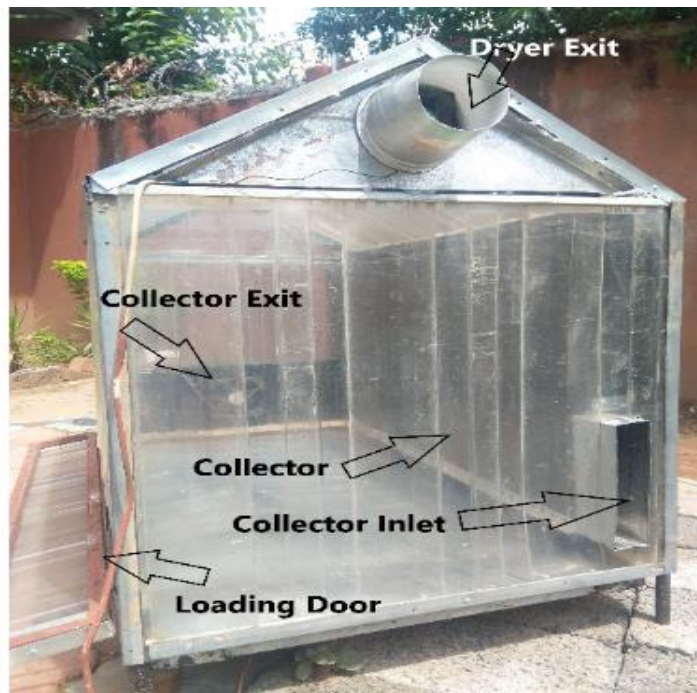
Figure 2. 17 GSD modified with a vertical solar thermal collector (Simate & Simukonda, 2022) Eltawil et al., (2018) developed a tunnel type dryer coupled with flat-plate collector and PV panels. Peppermint was dried inside the dryer in one, two, and three layers for evaluating dryer performance. The maximum drying time was 360 minutes inside the dryer while 420 minutes was under the open sun. The use of a thermal curtain gave better quality mint as compared to drying under the open sun. The dryer was reported to have an efficiency of 30.71%. Figure 2.18 below shows the GSD modified with a flat-plate solar thermal collector and PV module.
