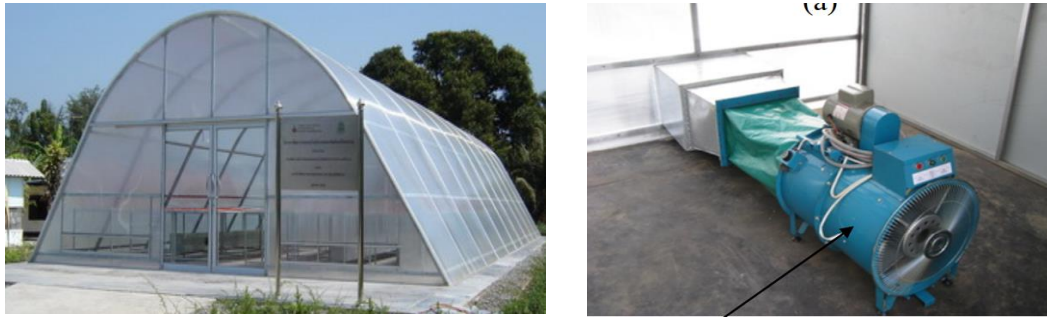
Figure 2. 26 GSD modified with a LPG burner (Janjai, 2012)
