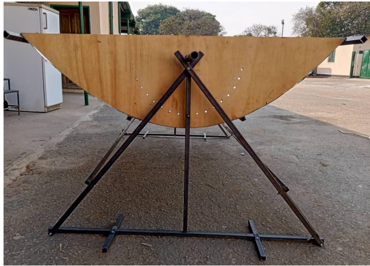
Figure 4. 2 Manual tracking system of the fabricated PTSC
