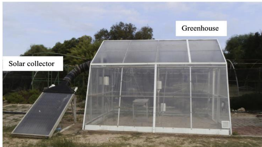
Figure 2. 19 GSD modified with a flat plate solar thermal collector (ELkhadraoui et al., 2015)
