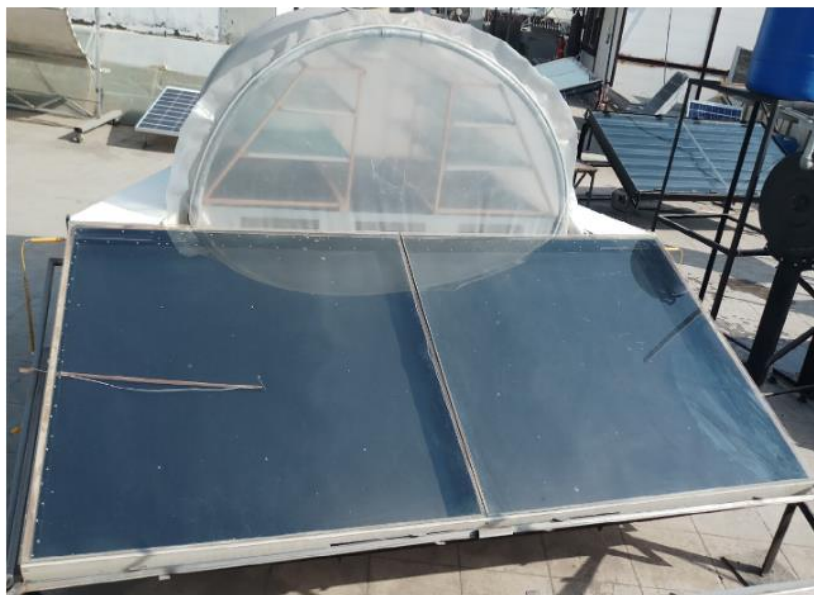
Figure 2. 20 GSD modified with flat plate collectors (Mehta et al., 2018)
