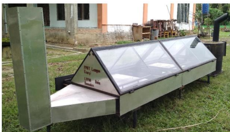
Figure 2. 23 GSD modified with a biomass burner (Hamdani et al., 2018)
