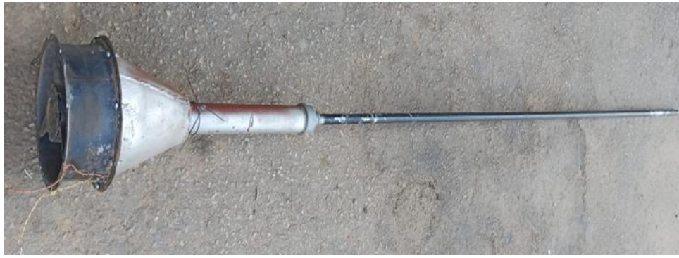
Figure 3. 5 Absorber tube connected to the axial fan
